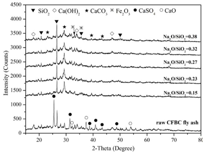
Figure 2. XRD analysis of CFBC fly ash based geopolymer (7 days)
