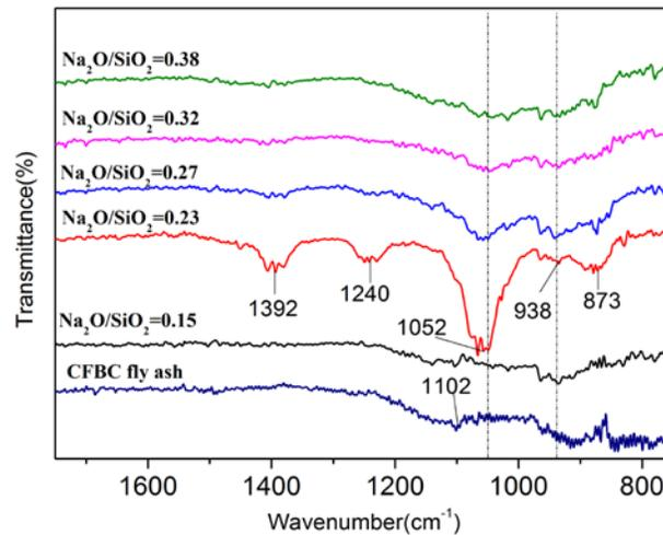
Figure 3. FTIR analysis of CFBC fly ash based geopolymer (7 days)
