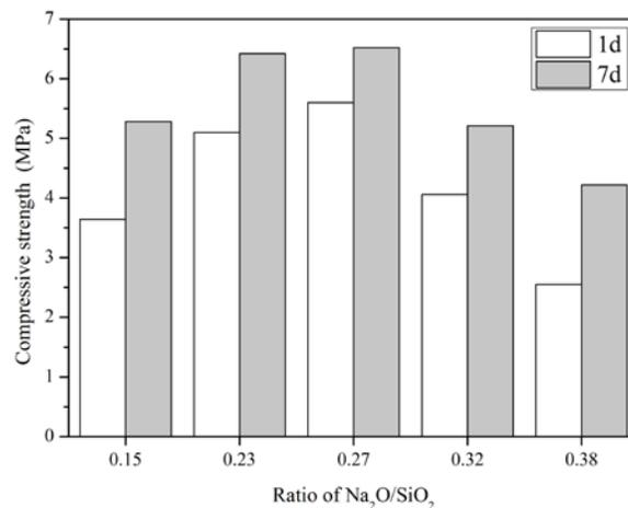
Figure 1. Compressive strength of CFBC fly ash based geopolymer
