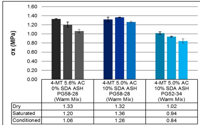
**FIGURE 8 The Horizontal Tensile Stress (MPa) at the Center of the Specimen**
