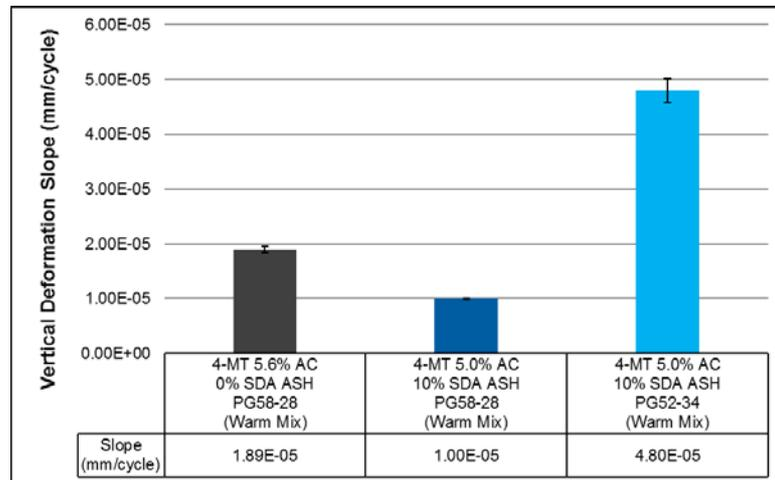
**FIGURE 11: The Vertical Deformation Slope (mm/cycle) for 4-MT WMA**
