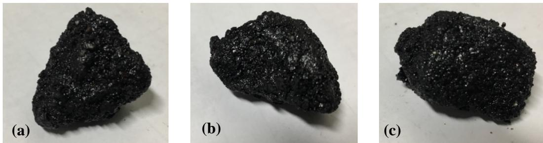
**FIGURE 4: Aggregate Coating (a) 4-MT WMA Control (b) 4-MT WMA ASHphalt (c) 4-MT WMA ASHphalt (PG52-34)**
