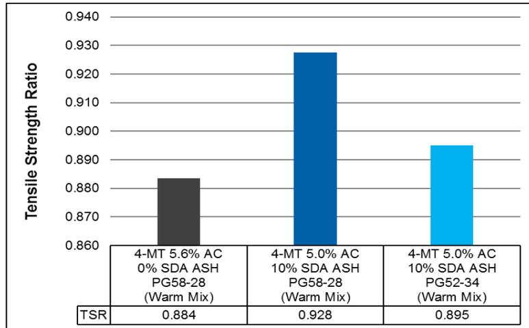
**FIGURE 10: Tensile Strength Ratio for all Mixtures**
