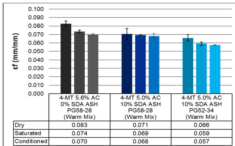
**FIGURE 9: The Horizontal Tensile Strain (mm/mm) at Failure**
