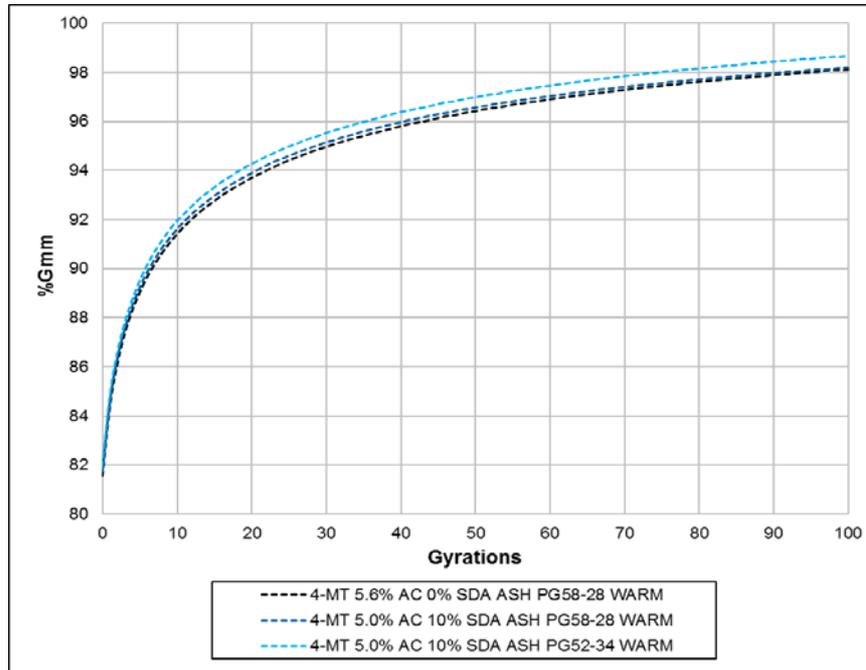
**FIGURE 5: The Densification Curve for 4-MT WMA**
