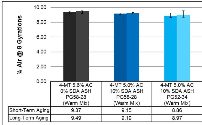
**FIGURE 6: The Air Content at 8 Gyration for 4-MT WMA**
