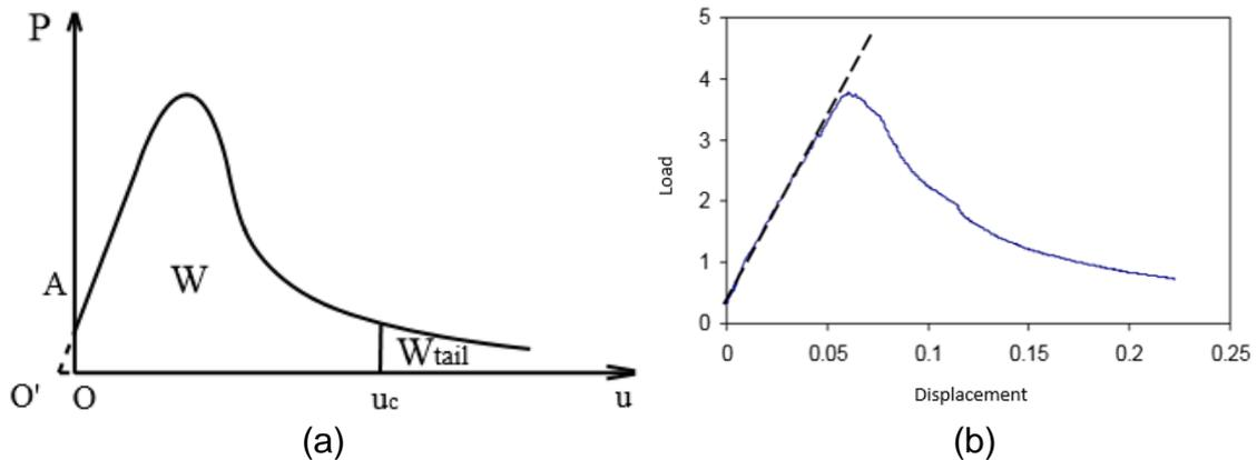
**FIGURE 3: (a) Low-Temperature Load vs. Load-Line Displacement Representation (b) Stiffness (S) Determination of Low-Temperature Testing**
