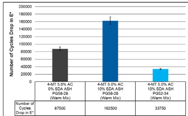
**FIGURE 12: The Number of Cycles to 50% Drop in E\* for 4-MT WMA**
