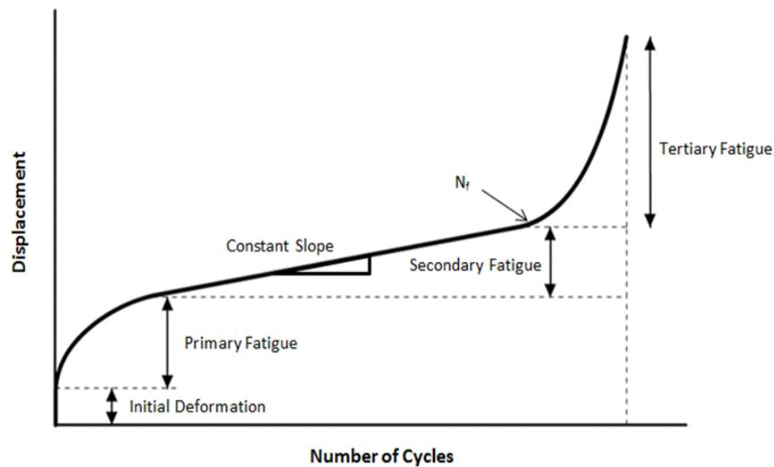
**FIGURE 2: Typical Deformation Plot for Repeated Fatigue Loading**
