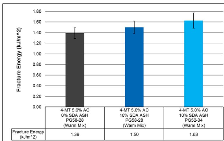
**FIGURE 13: The Fracture Energy ( $G_f$ ) Values for all Mixtures**
