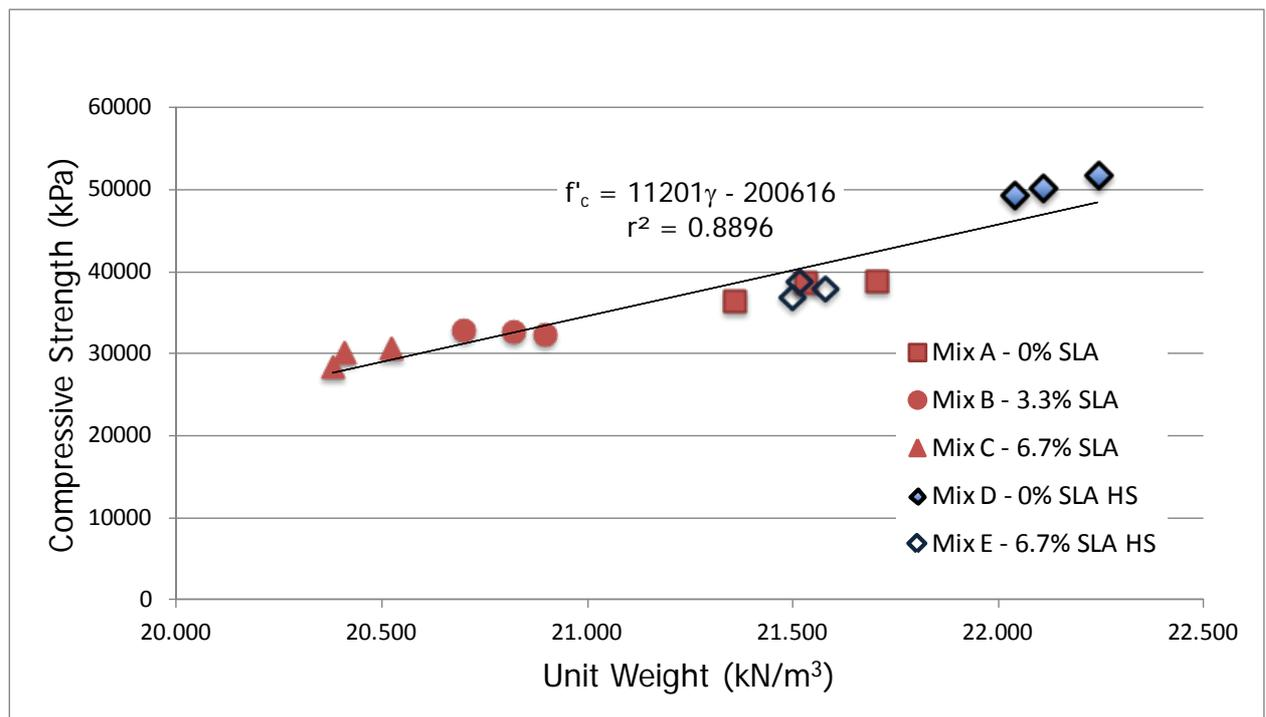
Figure 2 Compressive Strength Results for Various Mortar Concrete Tests Containing SLA
