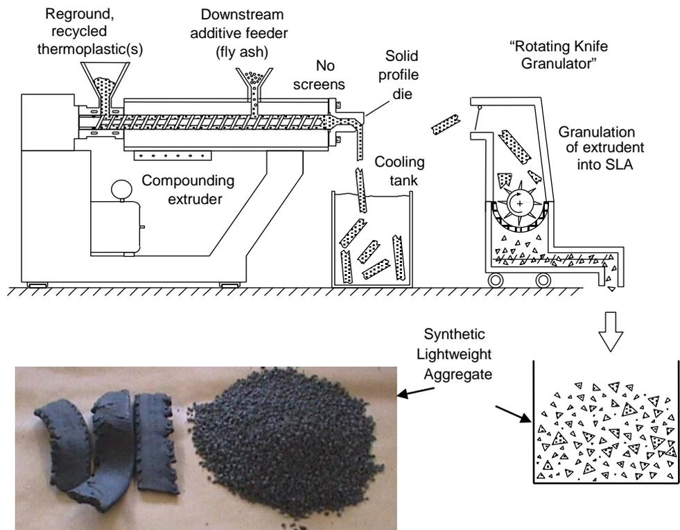
Figure 3 Schematic of SLA Production with Images of Extrudent (left) and Final Granulated Product (right)
