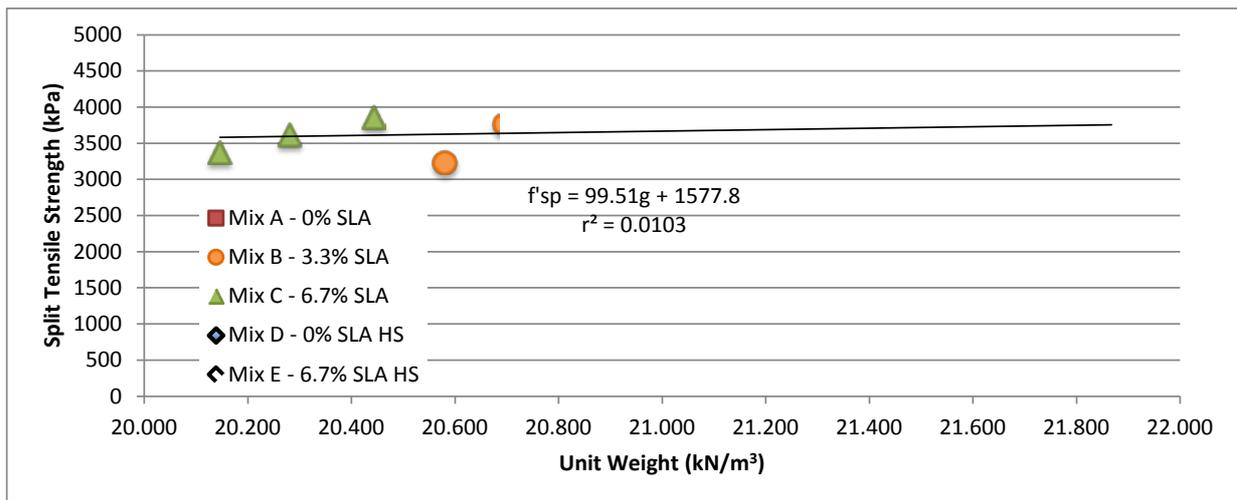
Figure 4 Split Tensile Strength Test Results for Various Mortar Concrete Tests Containing SLA
