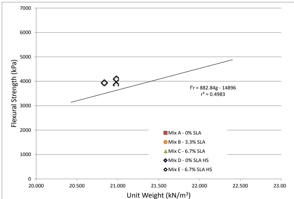
Figure 3 Flexural Strength Results for Various Mortar Concrete Tests Containing SLA
