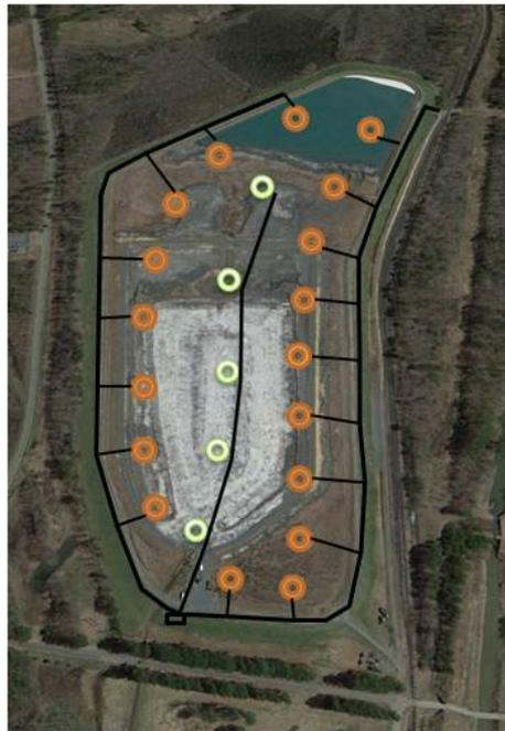
**Stage 3 - Production Dewatering** is the period where lowering the leachate level in the pond ash from the stabilized surface layer through the saturated deposit to the base of the pond. Duration can match leachate recovery rates with the plant's schedule for closure and leachate reuse to moisture condition new dry ash for landfill disposal.
