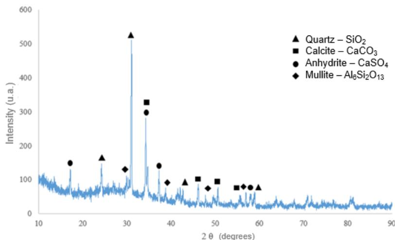
Figure 3 – AC-2 Diffractogram
