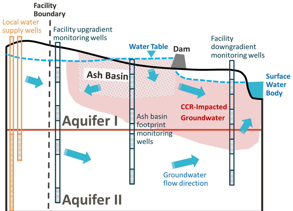
Figure 3: Schematic of the conceptual site model for the hypothetical scenario
