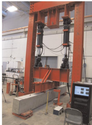
c) Splice test setup with specimen loaded
