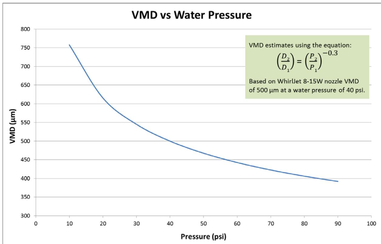
Figure 5 – Relationship between operating pressure vs droplet volume mean diameter (VMD) for WhirlJet 8-15W spray nozzle<sup>4</sup>
