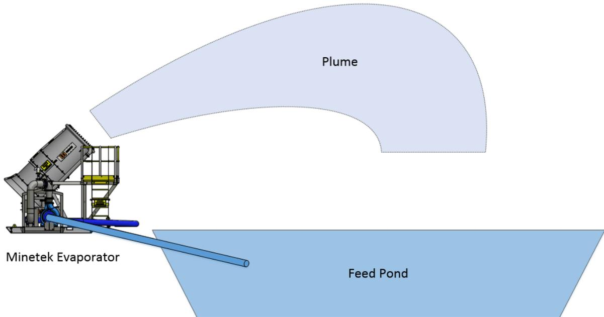
Figure 6 – Example of Minetek Evaporator operated in Closed –Loop configuration
