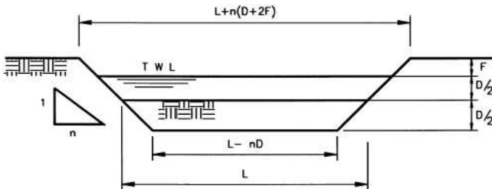
Figure 3 – Example of typical evaporation pond .design maximizing the top water surface<sup>3</sup>
