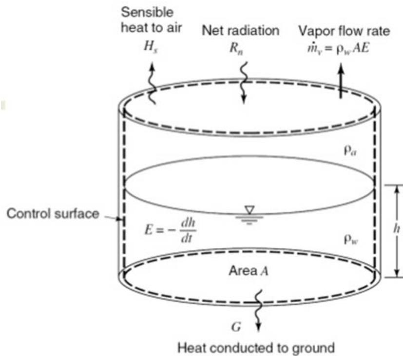
Figure 1 - Example of an evaporation pan model as applied to energy budget method of estimating evaporation rate<sup>1</sup>
