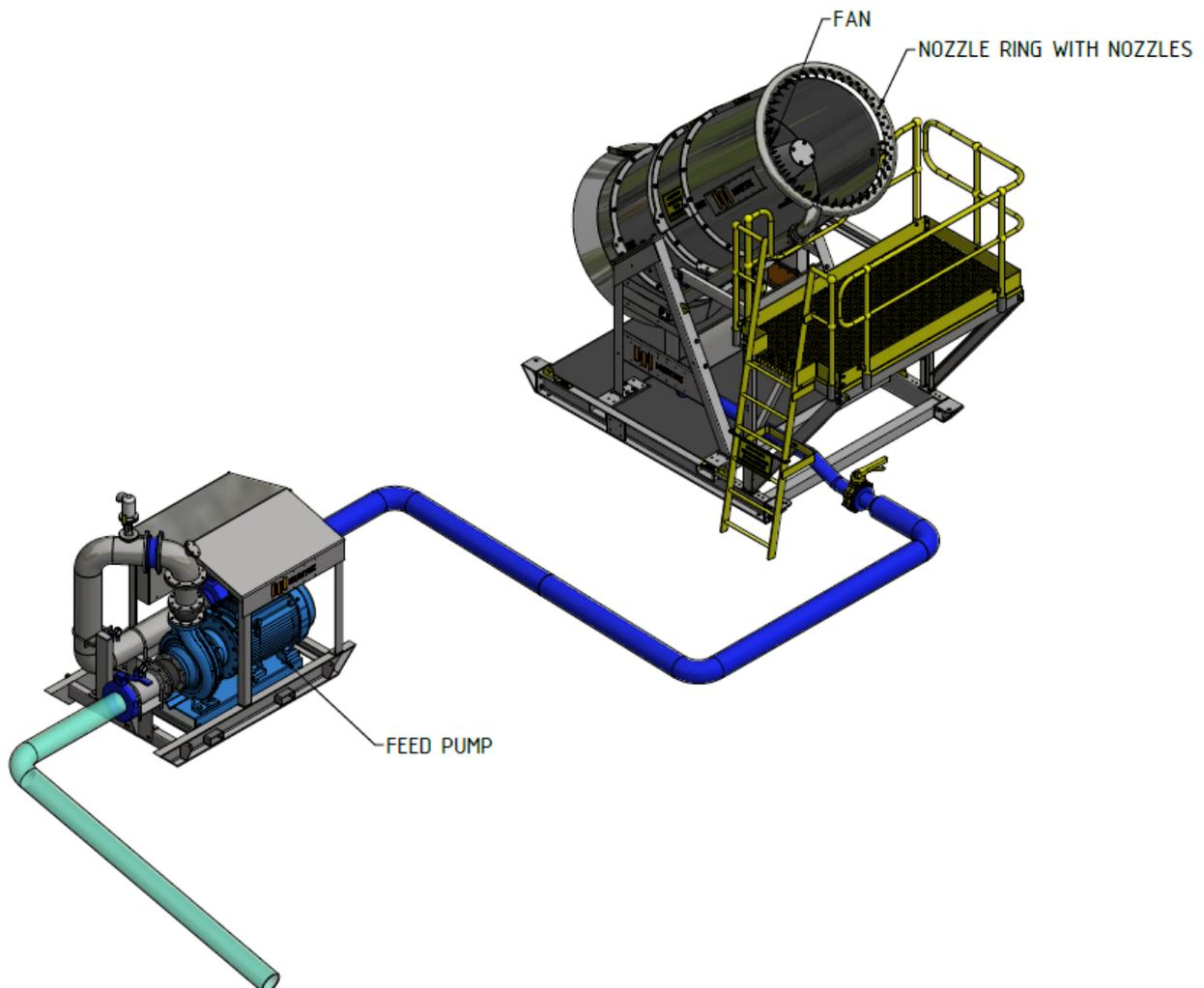
Figure 4 – The Minetek Evaporator
