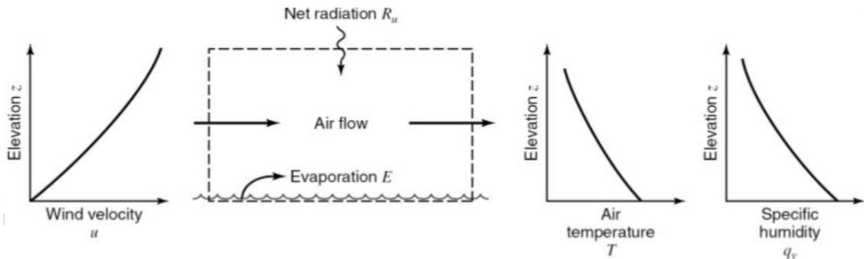
Figure 2 – Aerodynamic factors affecting evaporation of water from an open surface in relation to mass budget method of estimating evaporation rate<sup>1</sup>
