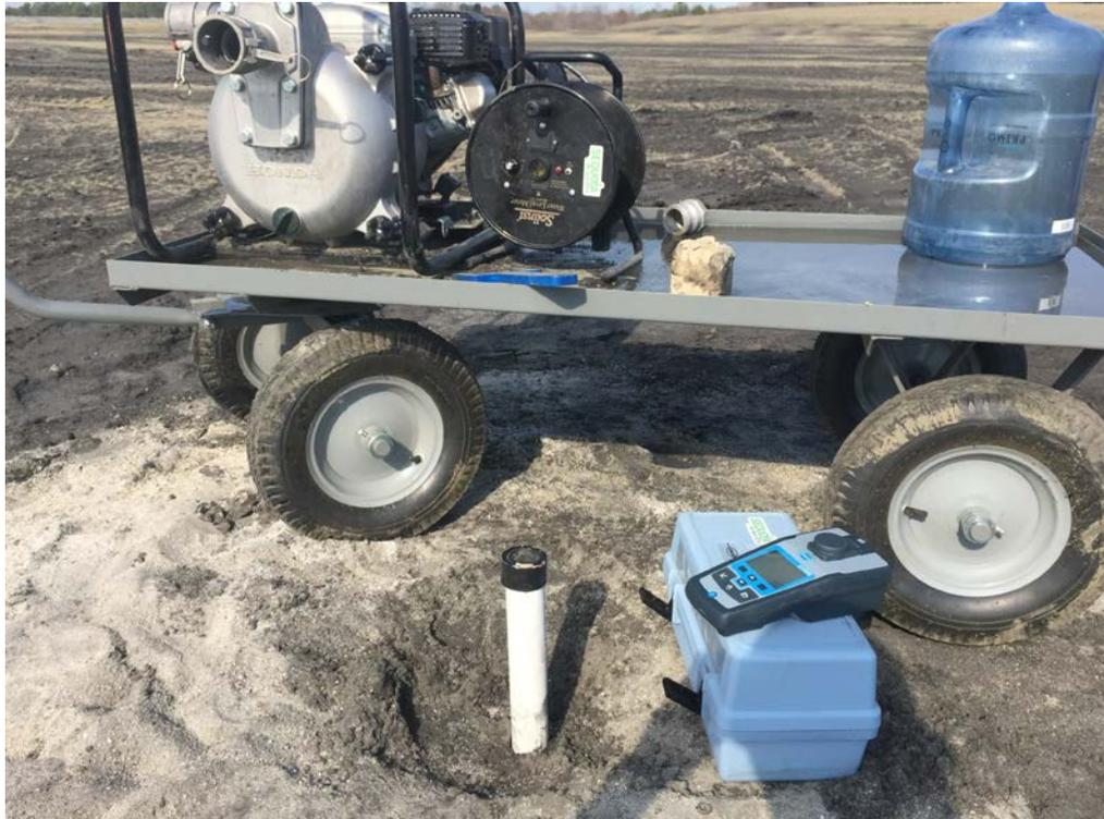
**Pictured: test cart with 2" contractor pump, water level indicator and turbidimeter preparing for wellpoint pilot testing. In the picture you will notice remnants of activated alumina media utilized to construct the filter pack.**
