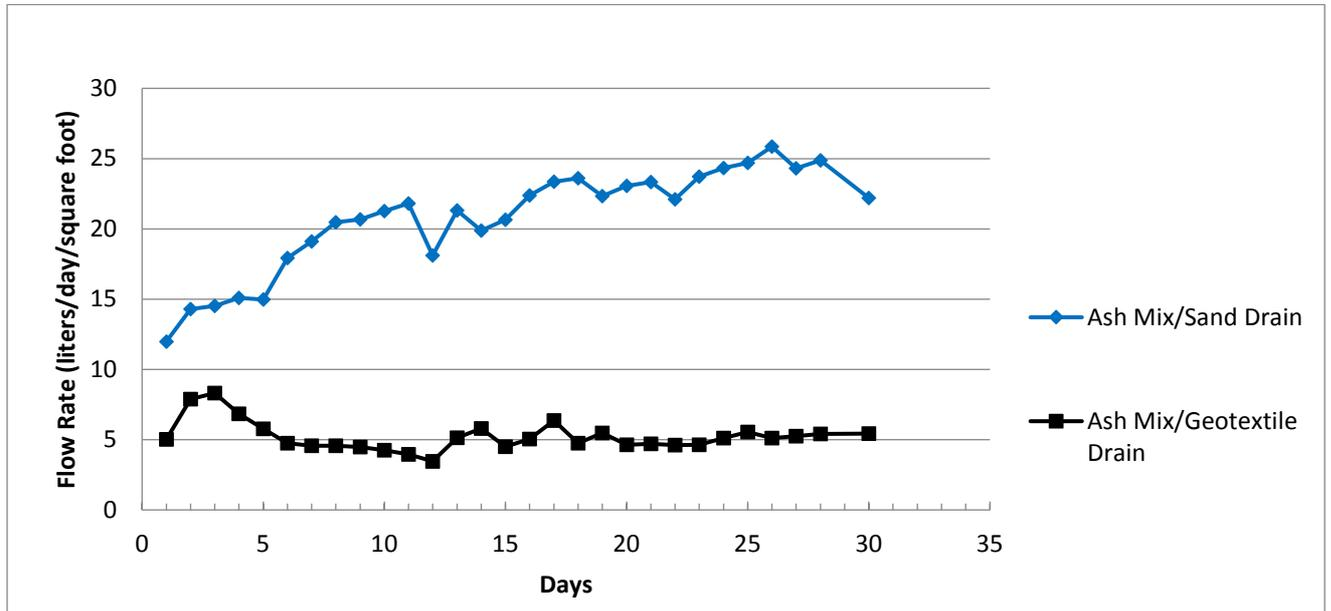
Figure 7. Flowrates through Ash Mixture Columns
