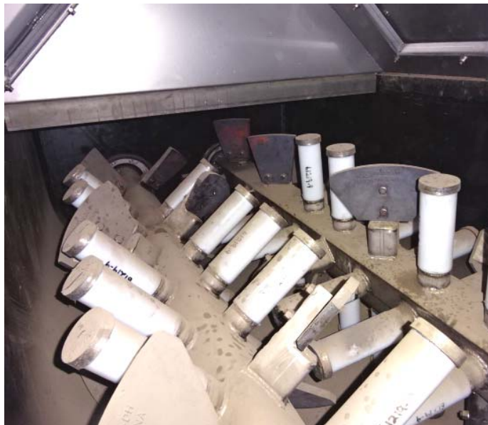
Photo 3. Corrosion Resistant Pin Paddle Mixer/Unloader
