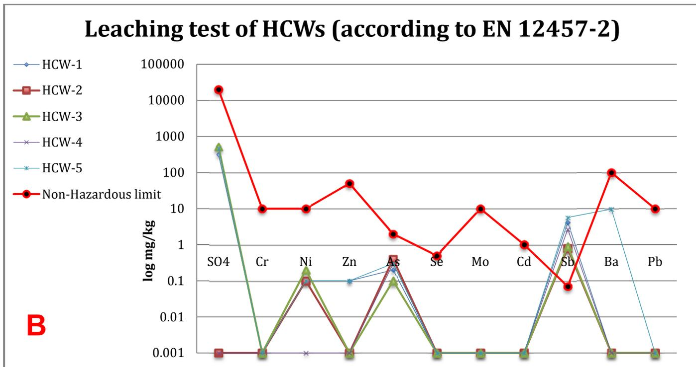
**Figure 5:** Leaching test according to the EN 12457-2 for aggregate products
