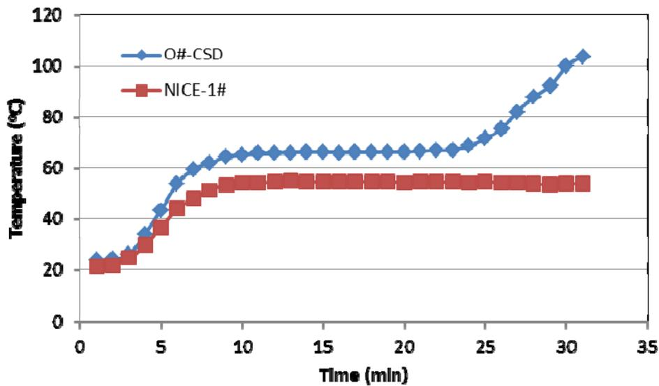
Figure 1 Temperature profiles of geopolymer foam vs. gypsum foam
