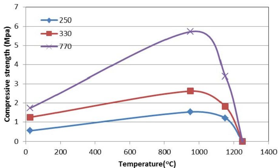
Figure 2 Compressive strength of geopolymer foams after 2-hrs at various temperatures
