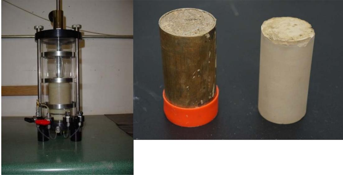
Figure 1: Permeability Cell and Test Cylinders
