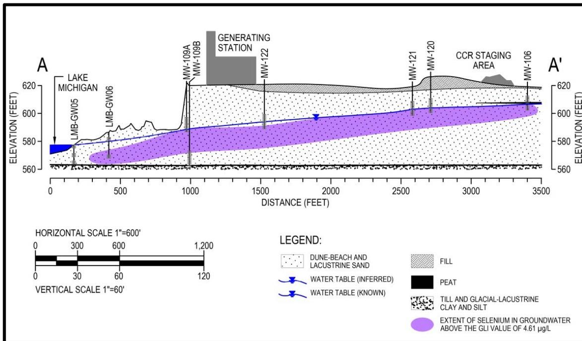
**Figure 7.** Extent of Selenium in the Surficial Aquifer – Cross Section
