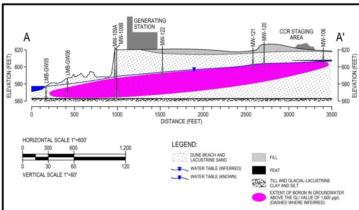
Figure 5. Extent of Boron in the Surficial Aquifer – Cross Section
