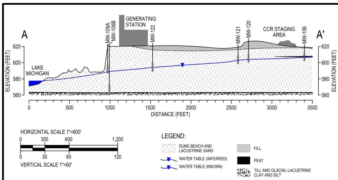
**Figure 2.** Geologic cross section showing shallow unconfined aquifer, CCR storage area and Lake Michigan
