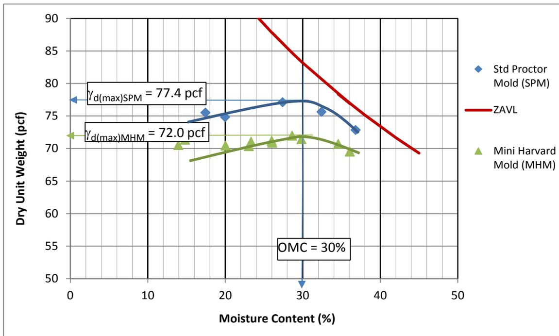
Figure 2: Density – Moisture Content Relationship of Site 1 CCRs Sample
