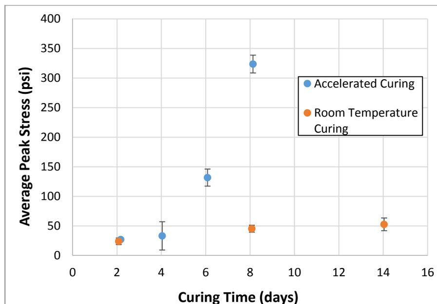
Figure 7: UCS of Site 1 Sample with 5 % Quick Lime Content
