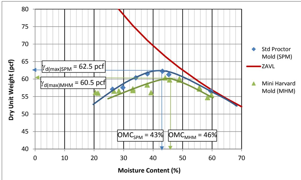
Figure 3: Density – Moisture Content Relationship of Site 2 CCRs Sample
