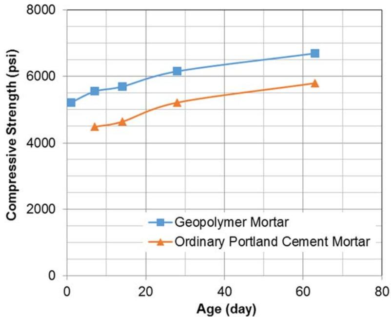
Figure 2: Comparison between geopolymer and OPC binders in 2-inch mortar cubes.
