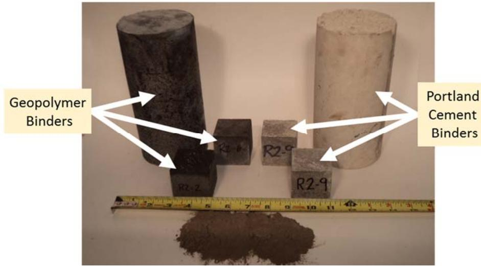
Figure 1: Geopolymer binders made from Carolina fly ash vs. OPC binders.
