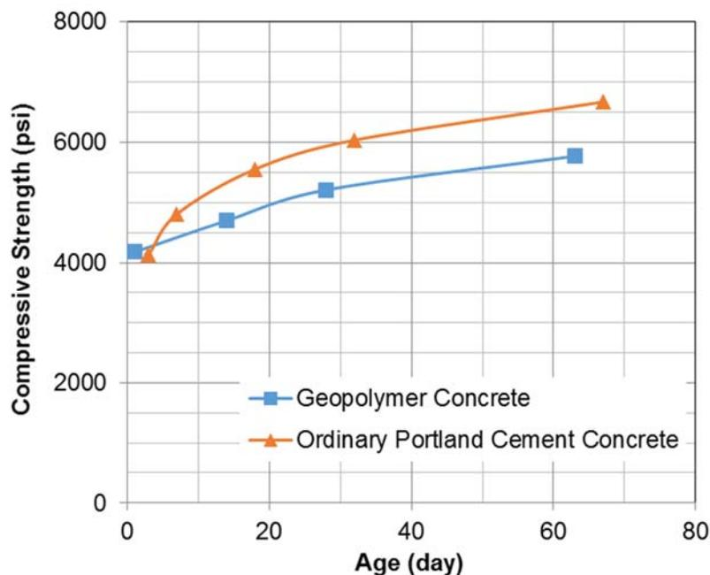
Figure 3: Comparison between geopolymer and OPC binders in concrete cylinders.
