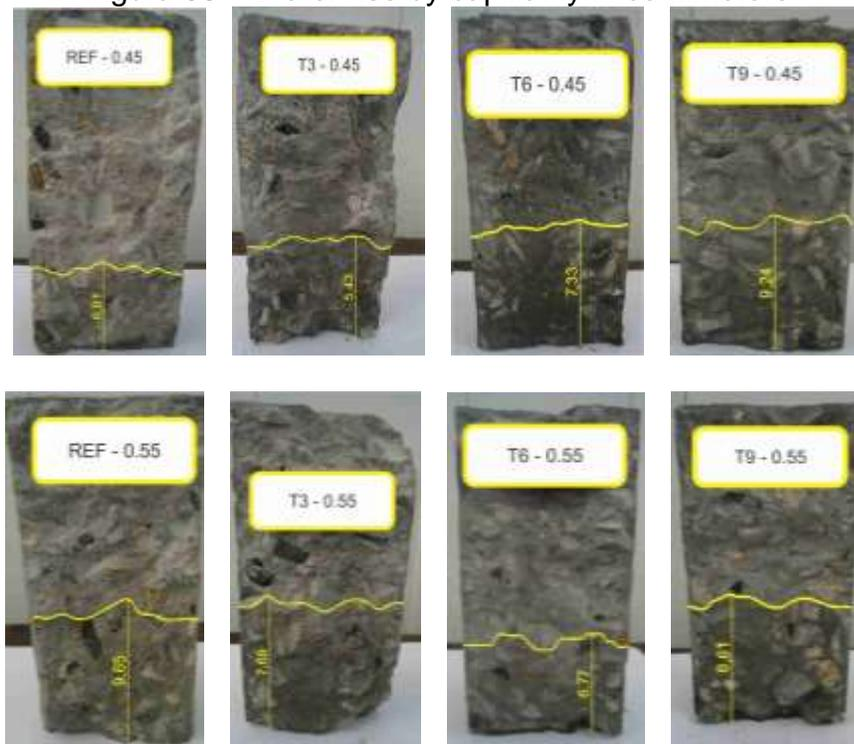
The reduction in water absorption and in water rise probably occurs due to precipitation of silicates generated by chemical reactions of coal ash with calcium hydroxide in larger voids of hardened paste, such as capillary channels<sup>2</sup>. However, this behavior does not appear in 0.45 w/c ratio mixtures.
