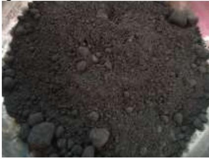
Figure 2 - 75µm sieved coal ash
