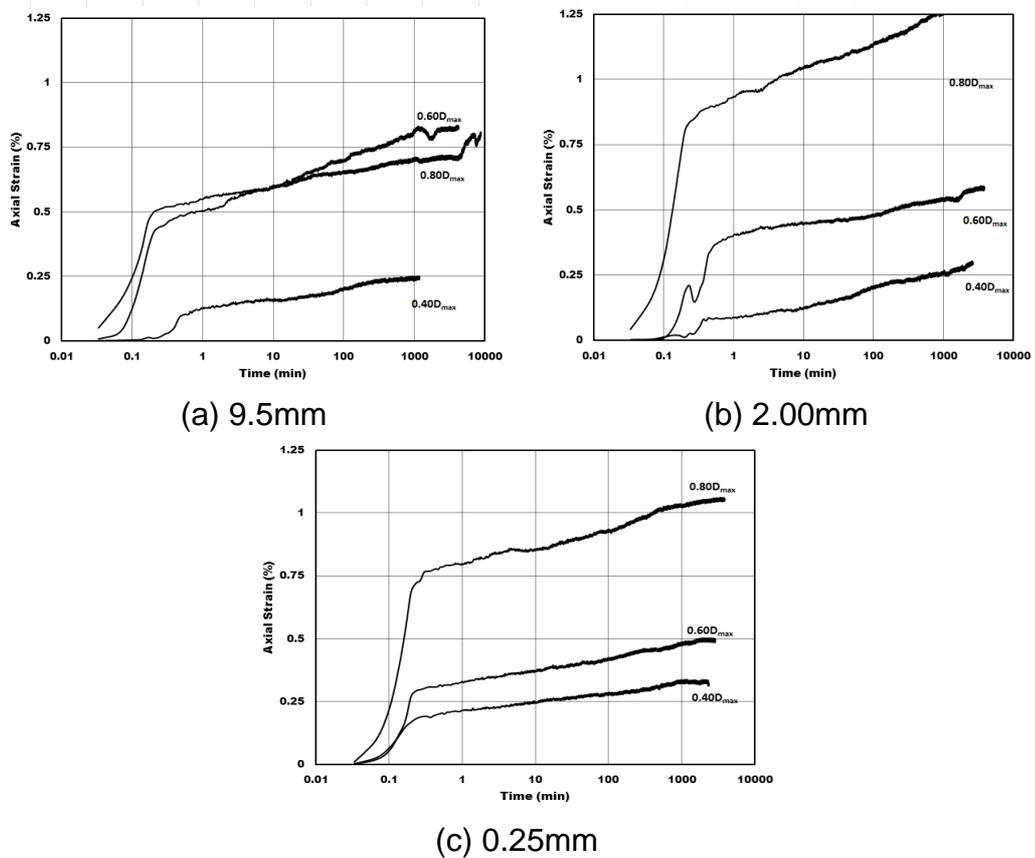
**Fig. 2 Relationships between Time and Axial Strain according to Maximum Grain Size**
