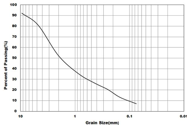
**Fig. 1 The particle size distribution curves of bottom ash**
