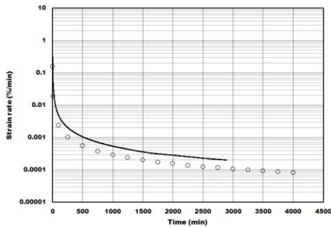
(c) Time vs Strain Rate (2.00mm)
