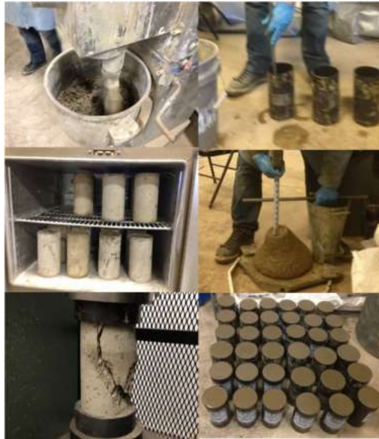
Fig. 2 (a) Mixing, (b) preparing cylinders, (c) curing, (d) measuring slump, (e) compressive strength test, (f) test specimens.
