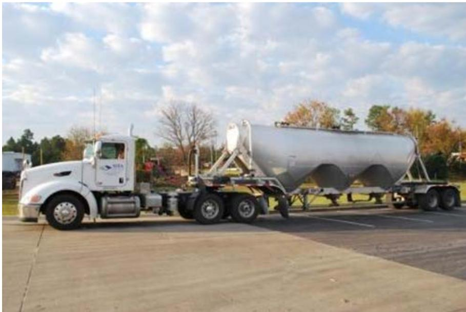
Figure 4 Fully Enclosed Fly Ash Transport Truck<sup>7</sup>
