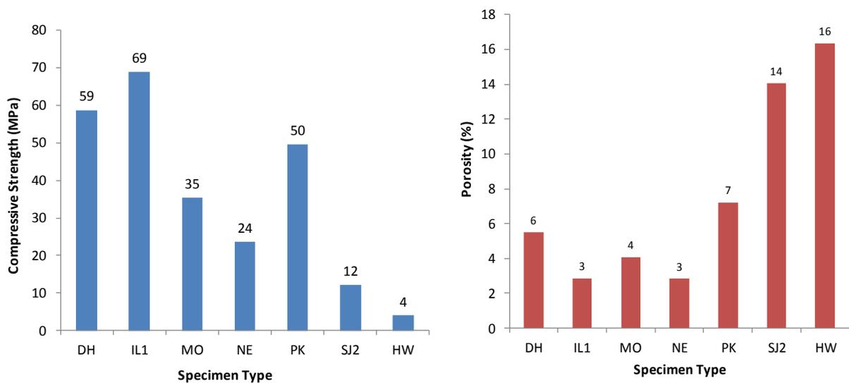
**Fig 1.** Compressive strength and porosity analysis of geopolymer concretes
