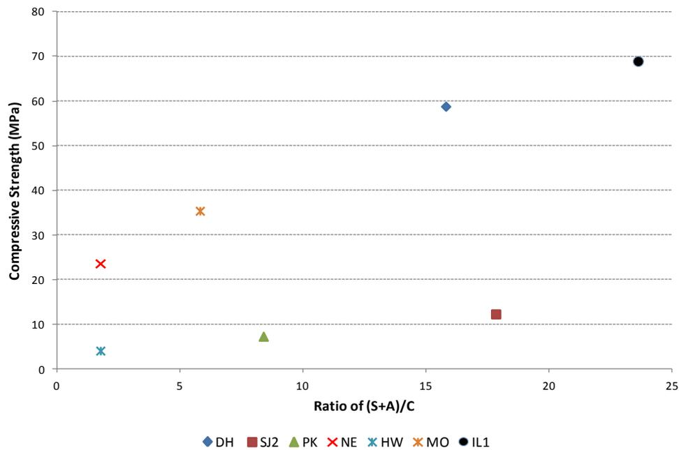
**Fig 2.** Ratio of  $(\text{SiO}_2 + \text{Al}_2\text{O}_3)/\text{CaO}$  versus compressive strength
