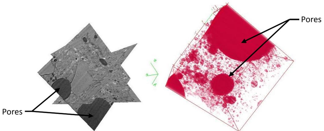
**Fig 6.** (a) Orthoslice image of GPC (MO), (b) 3D image exhibiting the pores
