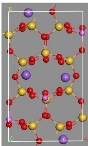
**Fig 8.** Optimized structure of Albite ( $\text{NaAlSi}_3\text{O}_8$ ) crystal structure, showing silicon (yellow), oxygen (red), aluminum (pink) and sodium (purple) atoms.
