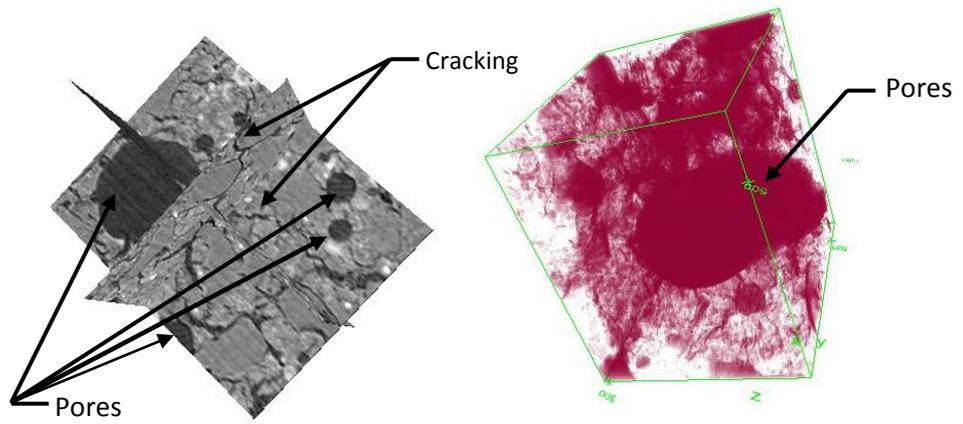
**Fig 5.** (a) Orthoslice image of GPC (HW), (b) 3D image exhibiting the large pores
