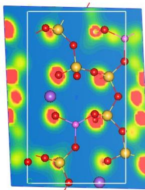
**Fig 10.** Electron Density Map of Albite as seen from the [001] direction
