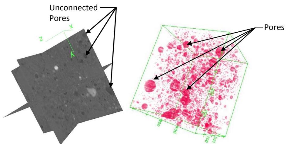
**Fig 7.** (a) Orthoslice image of GPC (IL), (b) 3D image exhibiting the pores
