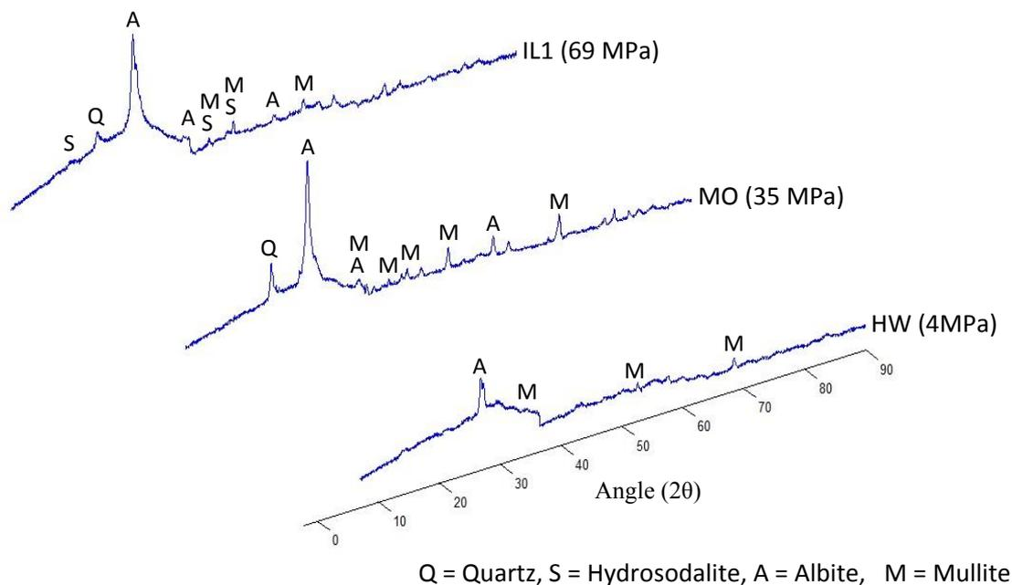
**Fig 4.** XRD analysis of low (4 MPa), medium (35 MPa) and high strength (69 MPa) geopolymer concretes
