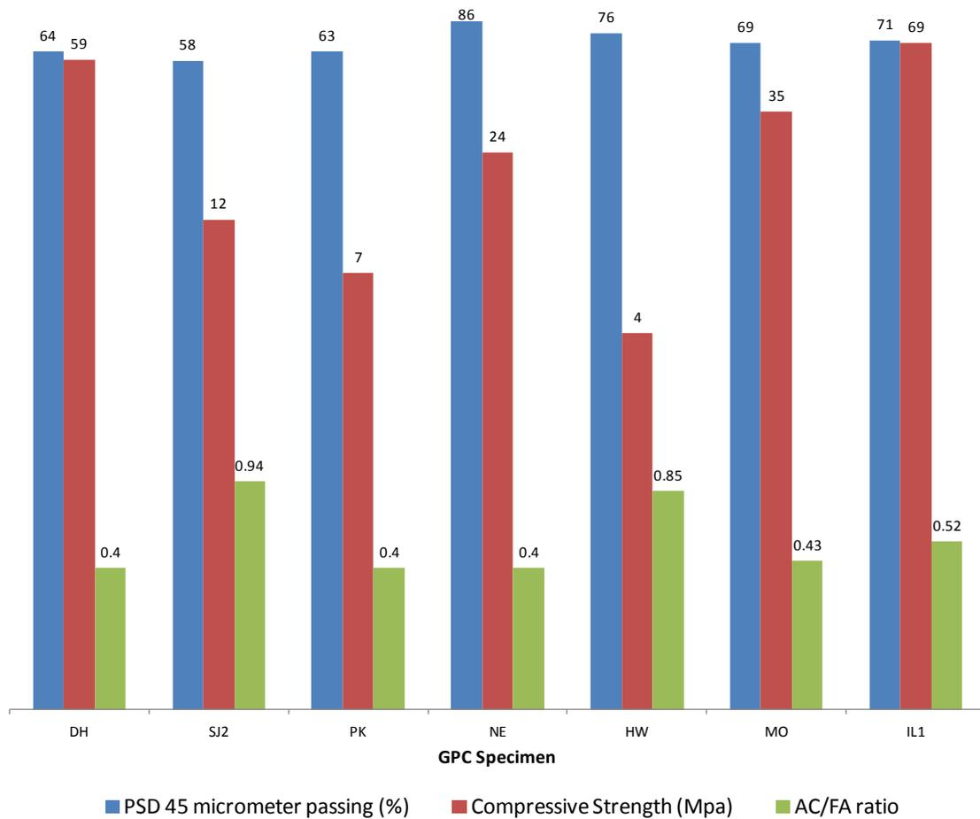
**Fig 3.** Relationship with Particle size distribution (PSD) and compressive strength of GPC
