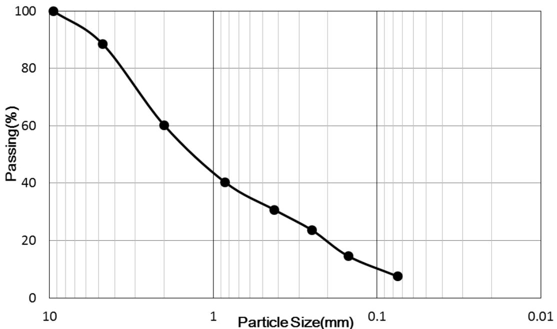
**Fig. 1** Particle size distribution of bottom ash(YH)
