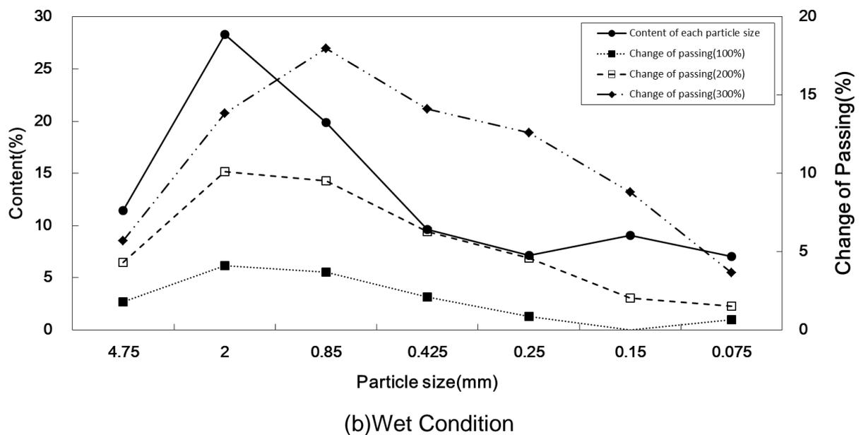
**Fig. 4** Content and change of passing ratio in each particle size
