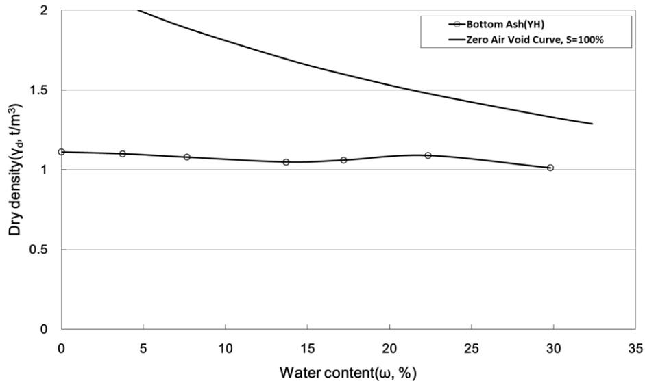
**Fig. 2** Compaction curve for YH bottom ash
