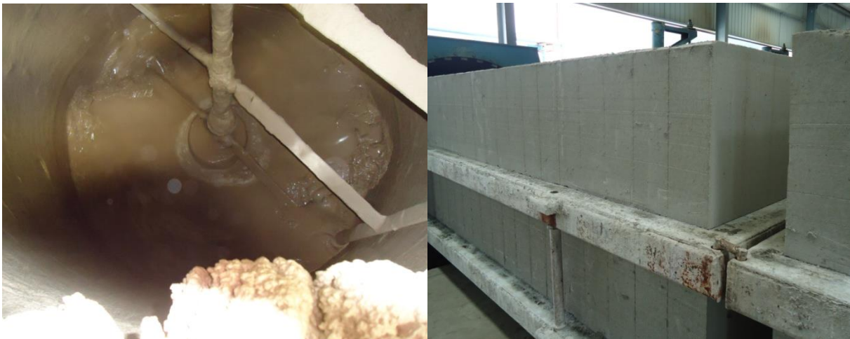
Figure 9 Autoclaved Aerated Concrete Production in HONGTAIXUN Pilot Plant
