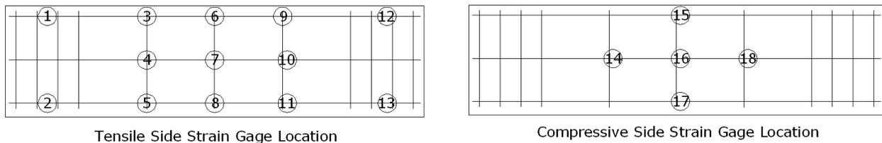
Figure 6. Strain Gage Schedule on the Rebars
