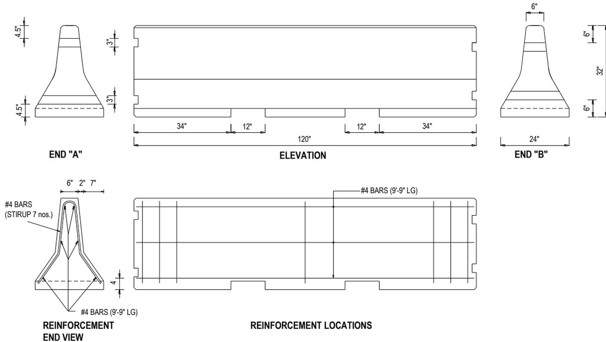
Figure 1. Schematic diagram of the median barrier (After Waskey Bridges Inc., *All dimensions are in inches unless specified otherwise*)
