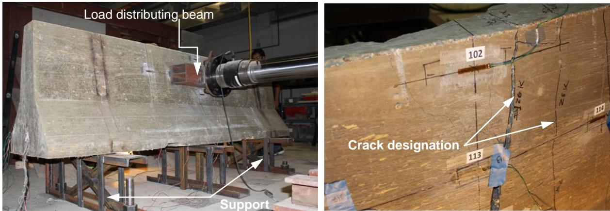
Figure 7. Barrier placed on bolted supports in front of the actuator (Left) and Crack designation and markings (Right).
