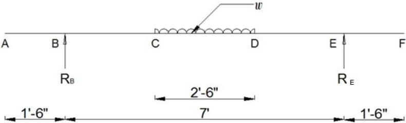
Figure 8. Free body diagram of the loading condition
