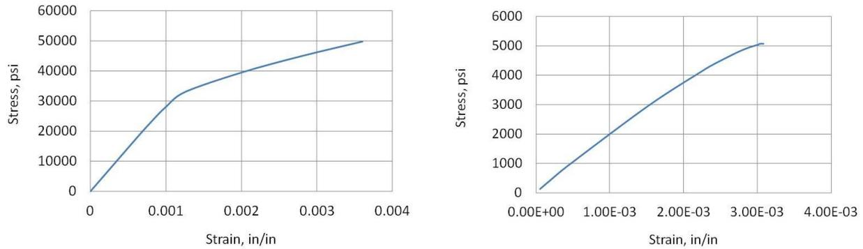
Figure 5. Stress-strain curves used for reinforcement steel (Left) and GPC (Right)
