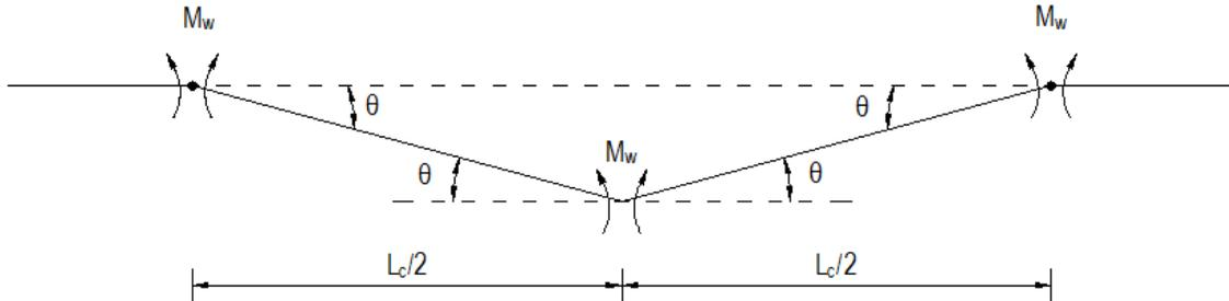
Figure 3. Plastic hinge mechanism for top beam as suggested by Calloway<sup>16</sup>
