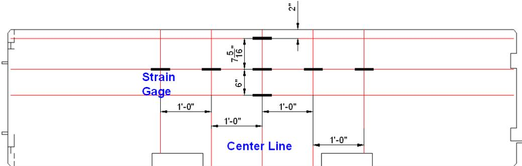
Figure 9. Location of strain gages placed on the surface of the GPC barrier
