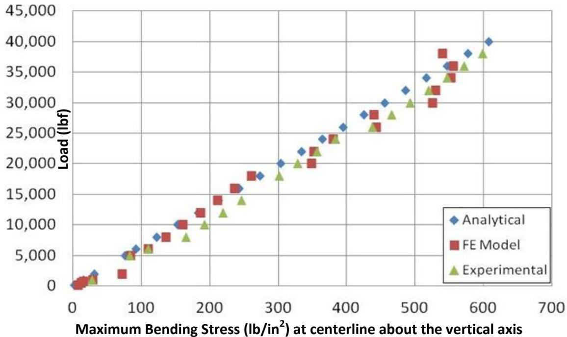
Figure 12. Comparison of obtained bending stress
