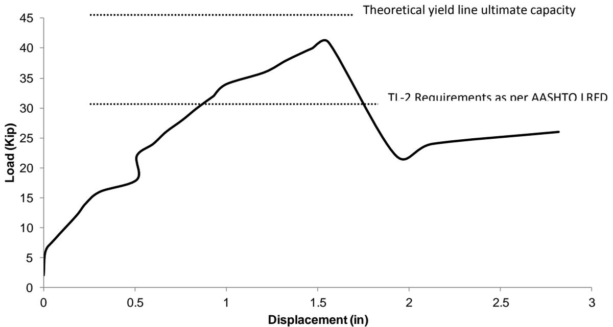
Figure 11. Experimental load displacement characteristics
