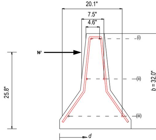
Figure 10. Sectional view showing the variation of effective depth for different rebars
