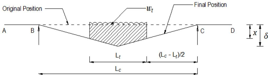
Figure 2. Original and deformed positions of the barrier wall<sup>16</sup>
