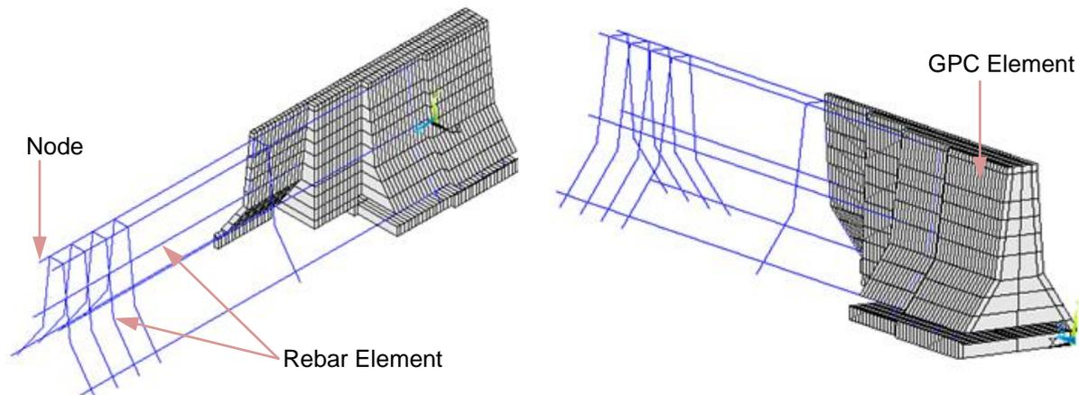
Figure 4. Simulation of concrete and steel elements
