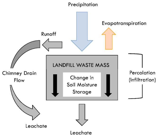
Figure 1: Leachate Generation Balance Diagram
