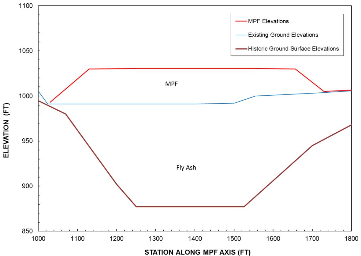
Figure 1 Cross-section across FAR 1 at the location of the MPF.
