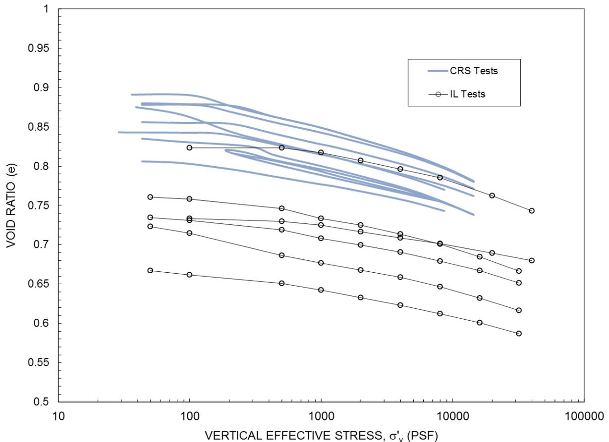
Figure 2  $e$ -log  $\sigma'_v$  for specimens consolidated using various reconstitution methods.
