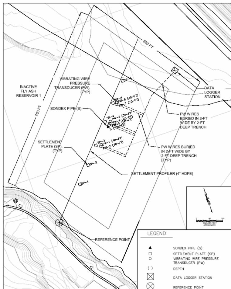
Figure 4 Geometry and Geotechnical Instrumentations of the MPF.
