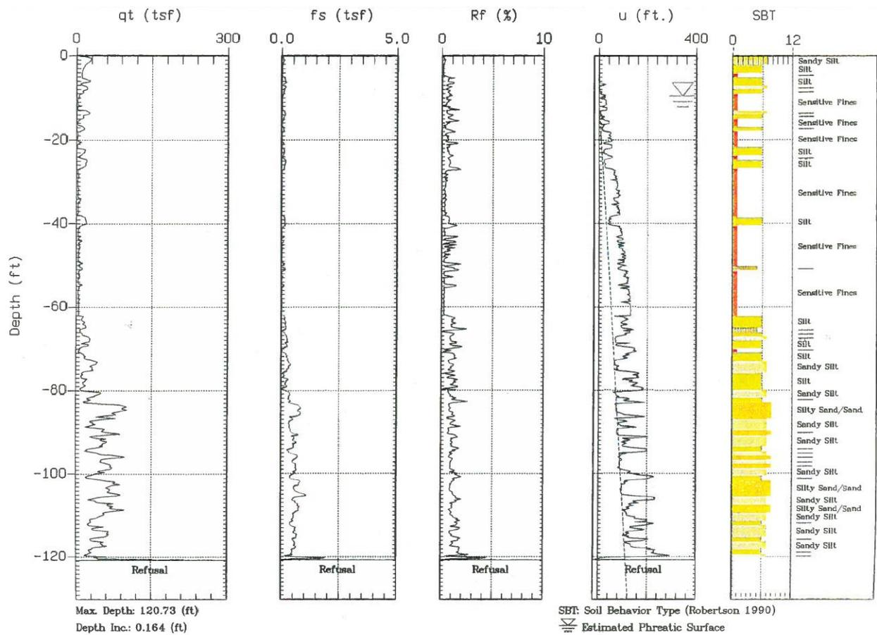
Figure 3 Typical results of the CPT in the vicinity of the MPF location.
