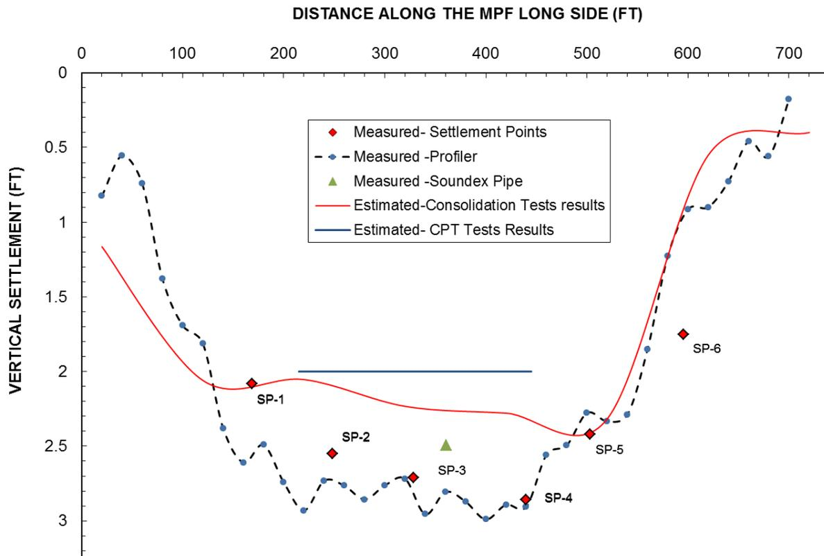
Figure 7 MPF Measured and Estimated Settlement
