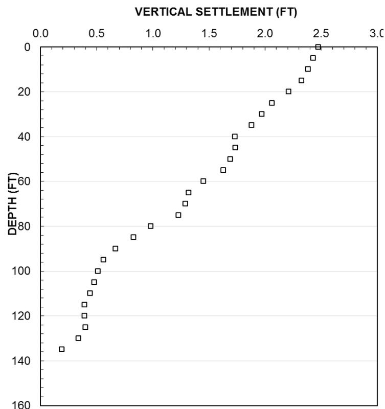
Figure 6 MPF Measured Settlement Using Soundex Pipe
