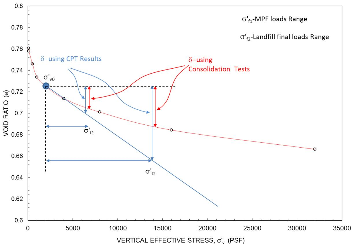
Figure 8 Illustration of Applicability of Field Measured Properties in Estimating Vertical Settlement.
