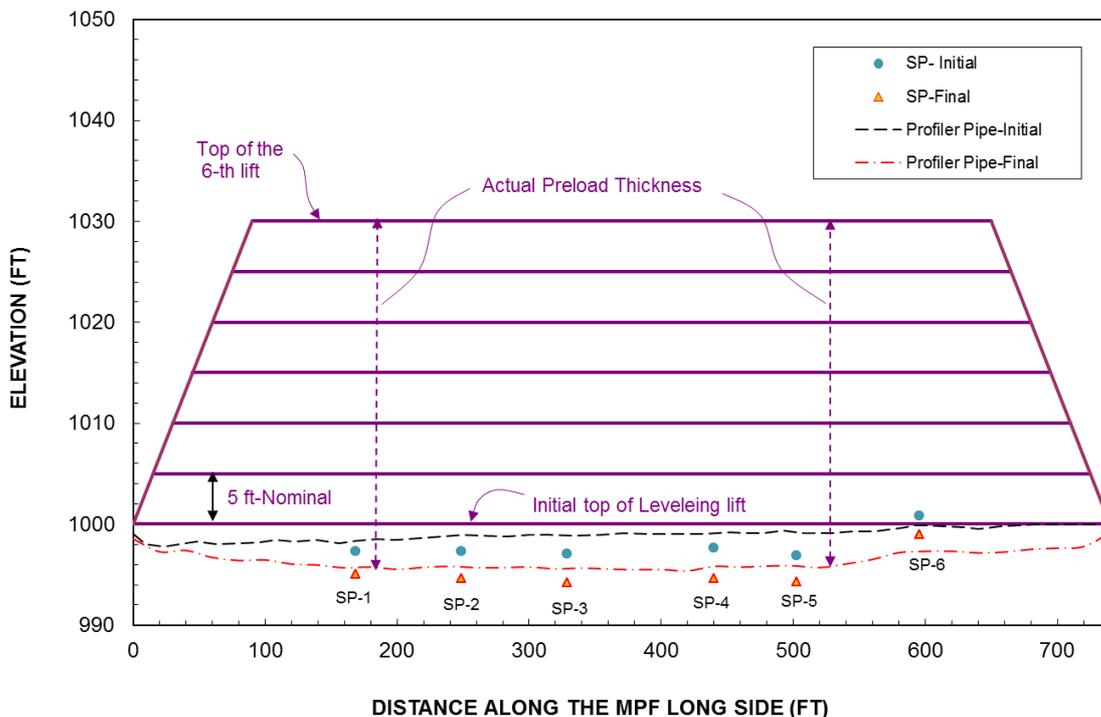
Figure 5 MPF Load Increments and Measured Settlement
