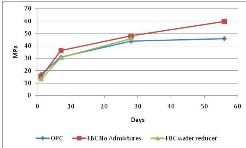
Figure 2. Mortar strength data for AR-FA with OPC I.
