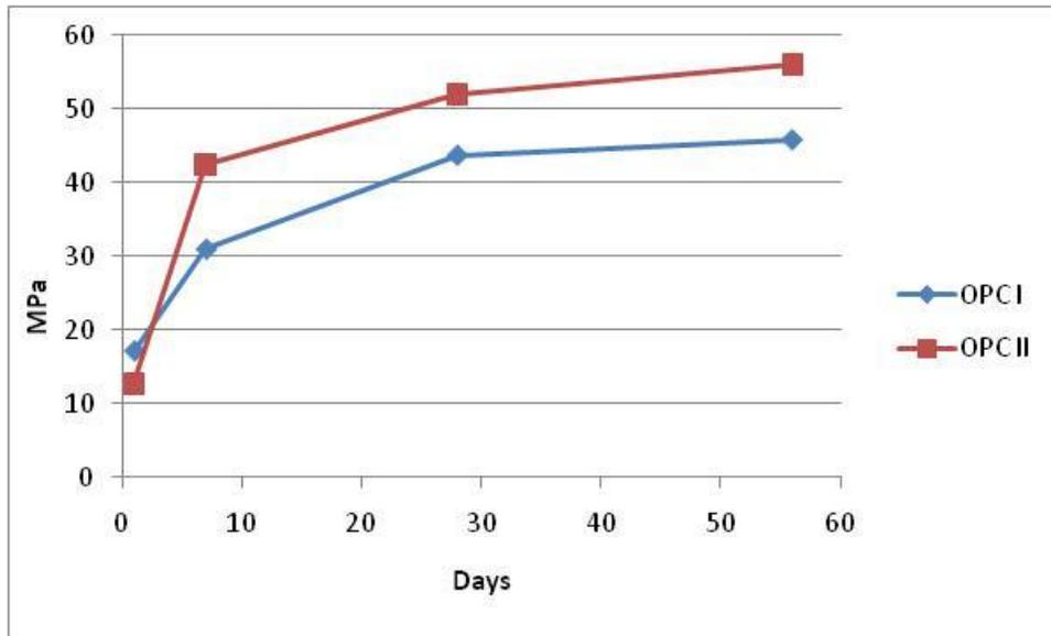
Figure 1. Plot of mortar strength development for the two OPCs used in the study.
