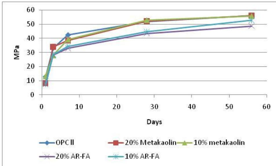
Figure 3. Mortar strength data for AR-FA and metakaolin with OPC II.
