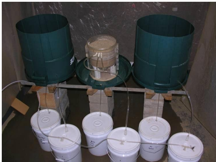
Figure 3 Cylinder and soil sample arrangement showing runoff and sediment collection systems used to evaluate FGD gypsum effects on erodibility using a rainfall simulator under laboratory conditions.
