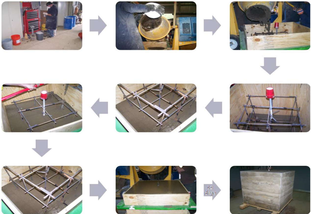
Figure 3. Sequential order of geopolymer concrete mixing, pouring, finishing and curing.
