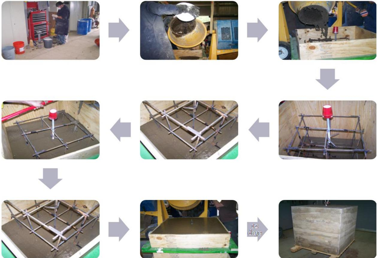
Figure 3. Sequential order of geopolymer concrete mixing, pouring, finishing and curing.
