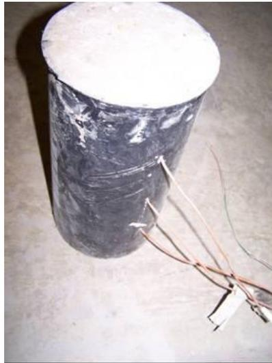
Figure 1. Geopolymer concrete cylinder with embedded thermocouples
