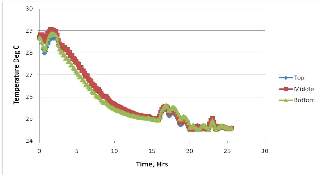
Figure 5. Temperature profile of Geopolymer Concrete Cylinder.
