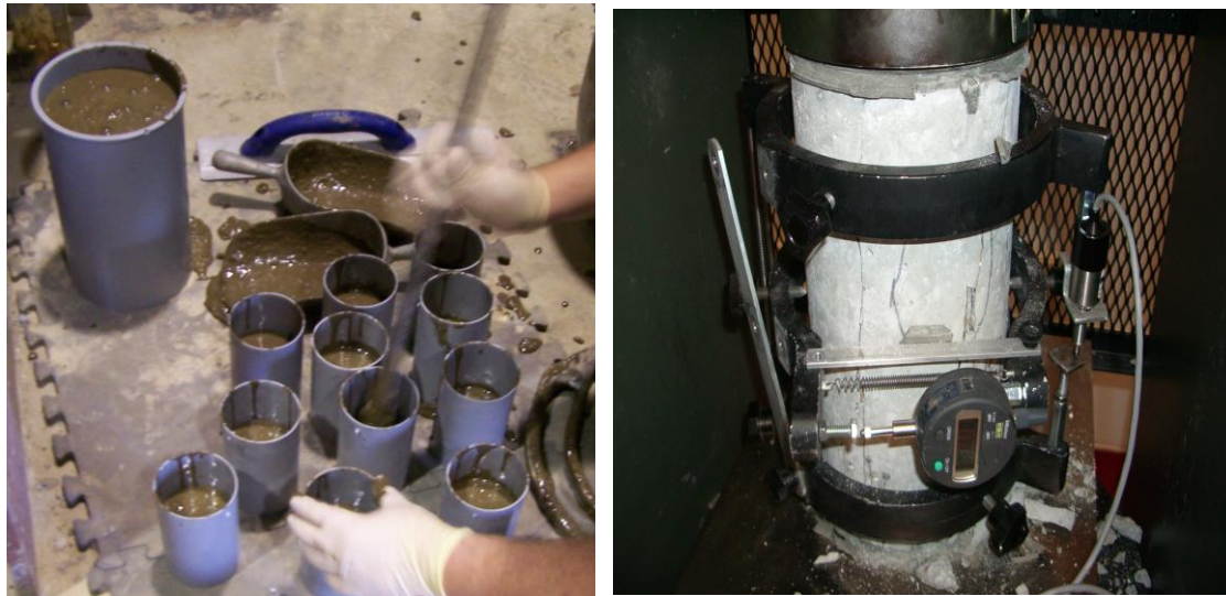
Figure 4. Pouring of cylinder samples and testing GPC cylinder.
