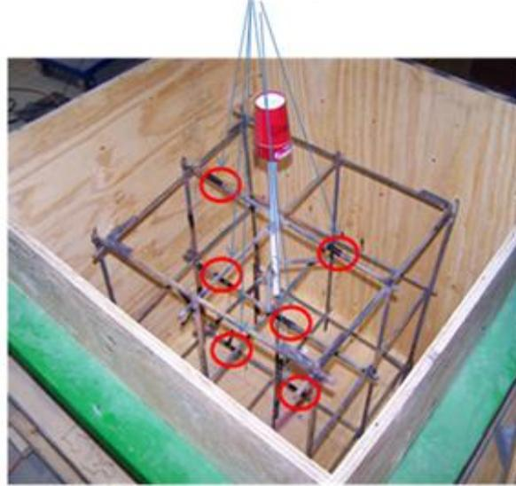
Figure 2. Wooden mold with steel reinforcement and thermocouples.
