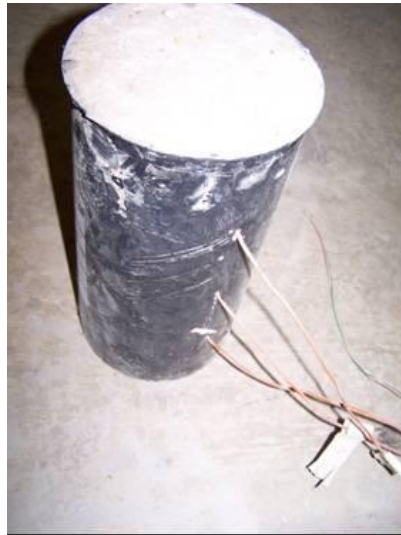
Figure 1. Geopolymer concrete cylinder with embedded thermocouples
