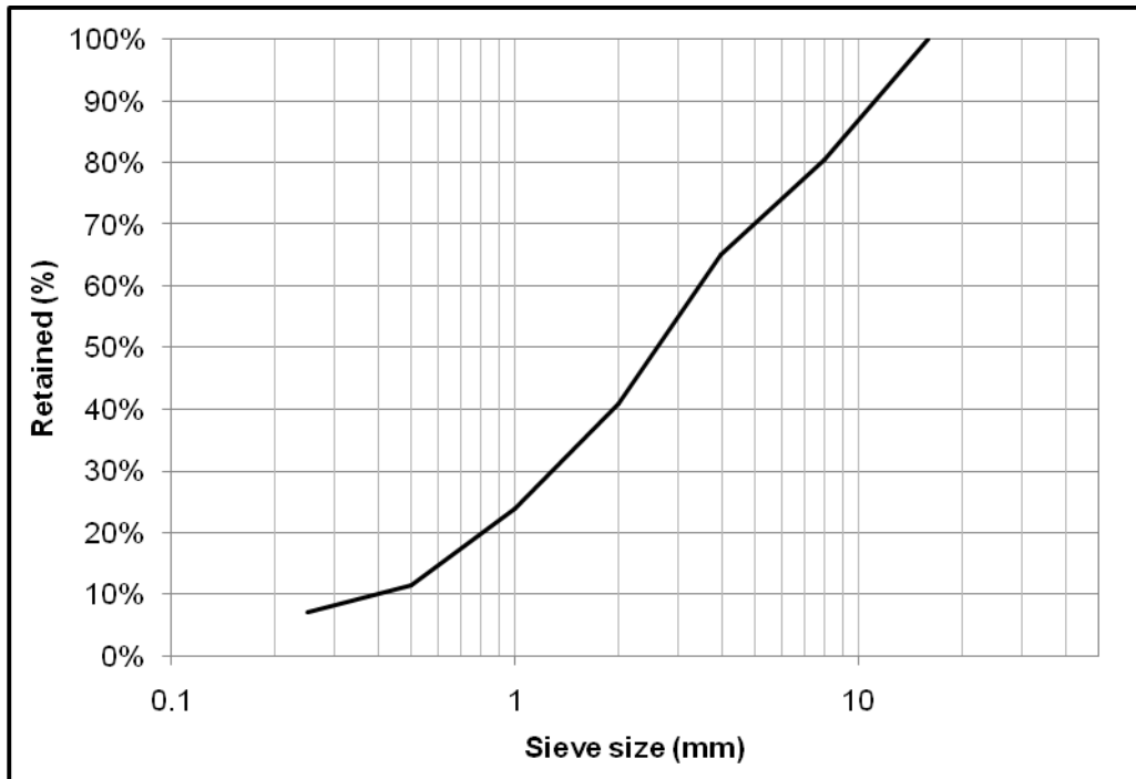
Fig. 1. Granulometry of aggregate mix used in all SCC mixtures
