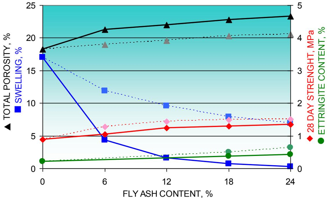
**Figure 11.** Relationship between porosity, swelling, strength, ettringite content and fly ash level in Lias clay (stabilized with 3% CaO, test age 7 days except for strength, FA1: broken lines, FA4: solid lines)
