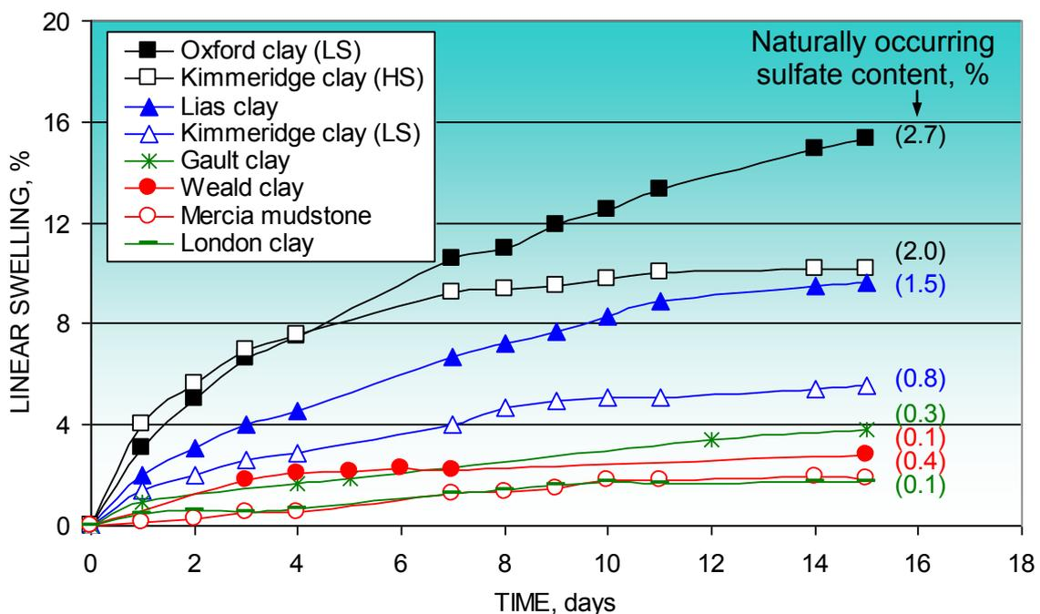
**Figure 1.** Linear swelling of lime-stabilized clays containing various sulfate levels (stabilized with 6%  $\text{Ca}(\text{OH})_2$ , no fly ash)
