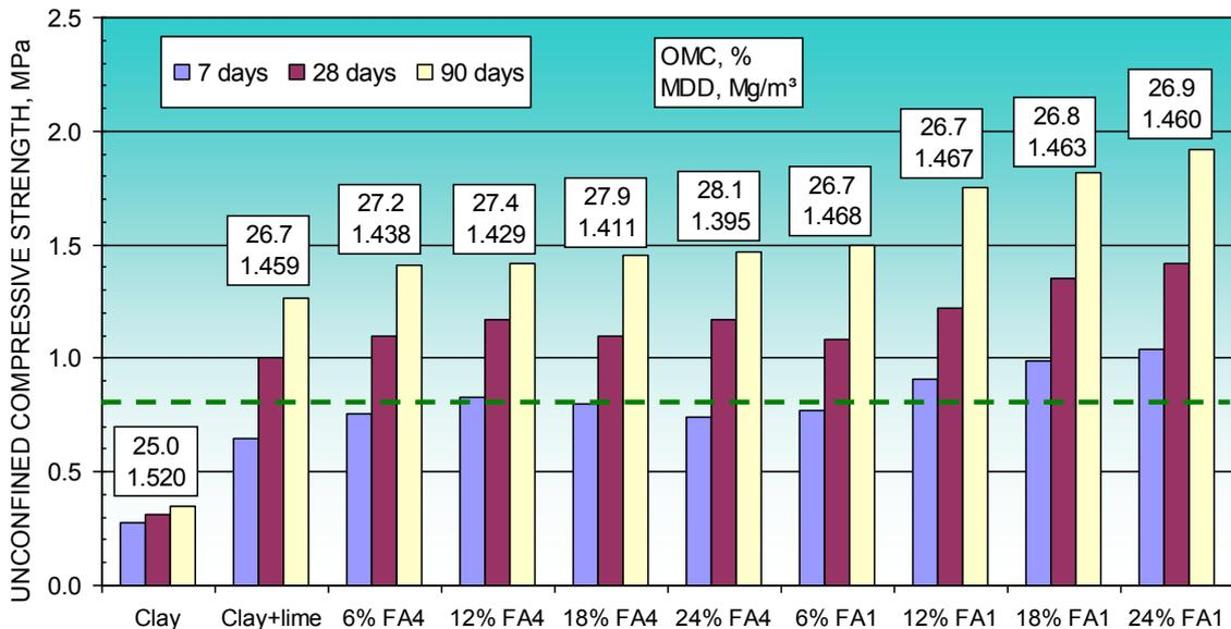
**Figure 4.** Strength gain of moist-cured Oxford clay specimens (stabilized by 3% CaO and 0 to 24% FA4 and FA1 fly ash)
