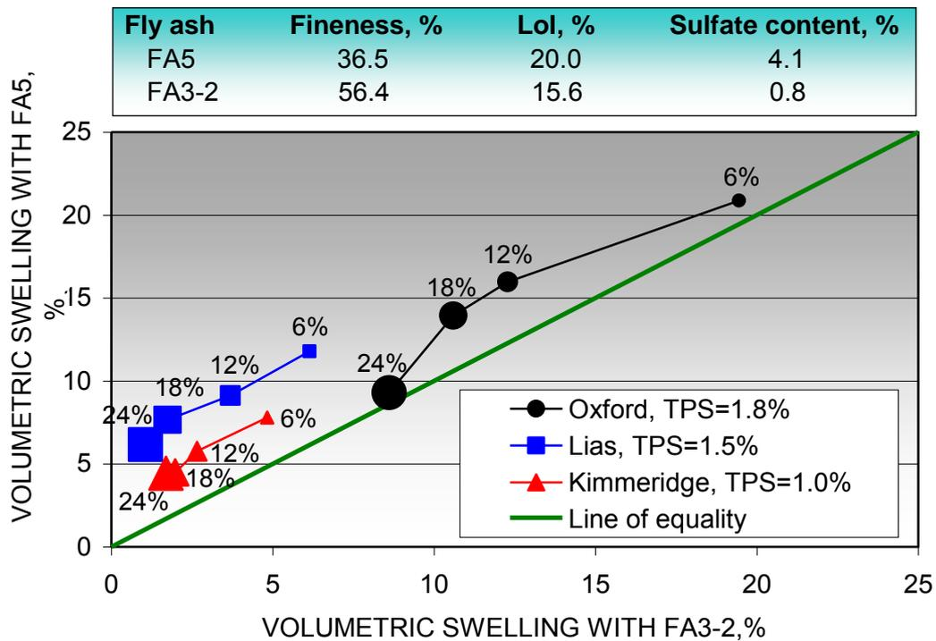
**Figure 8.** Effect of fly ash sulfate content and addition level on swelling of Oxford, Lias and Kimmeridge clays, (stabilized with 3% CaO)
