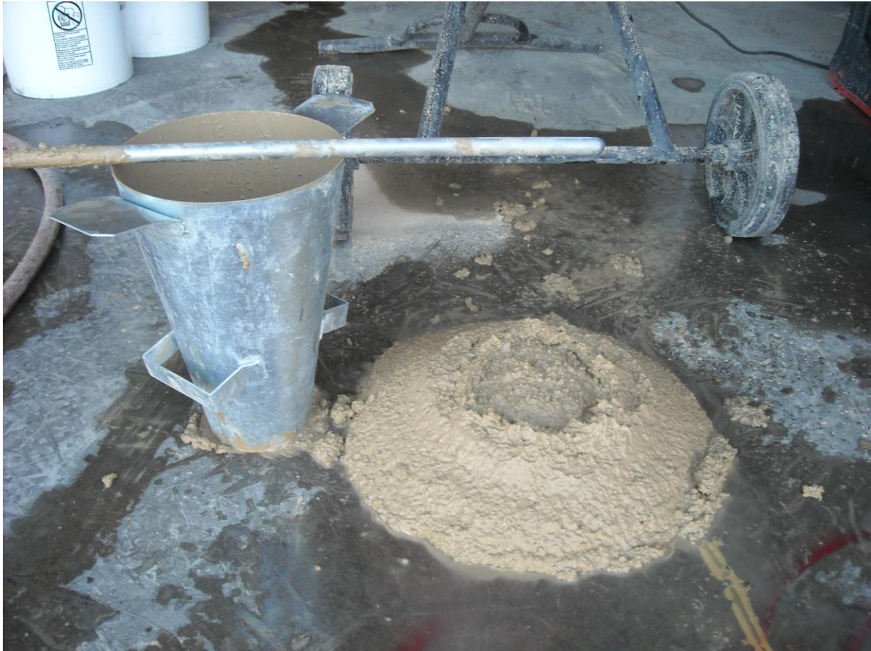
FlashCrete with 2200lb of Squeegee, with a more traditional-looking 9" slump
