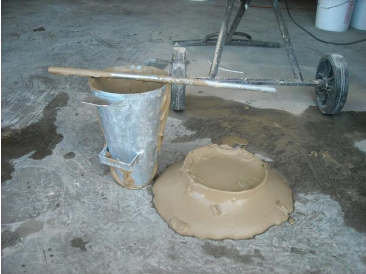
FlashCrete with a 9" Slump
