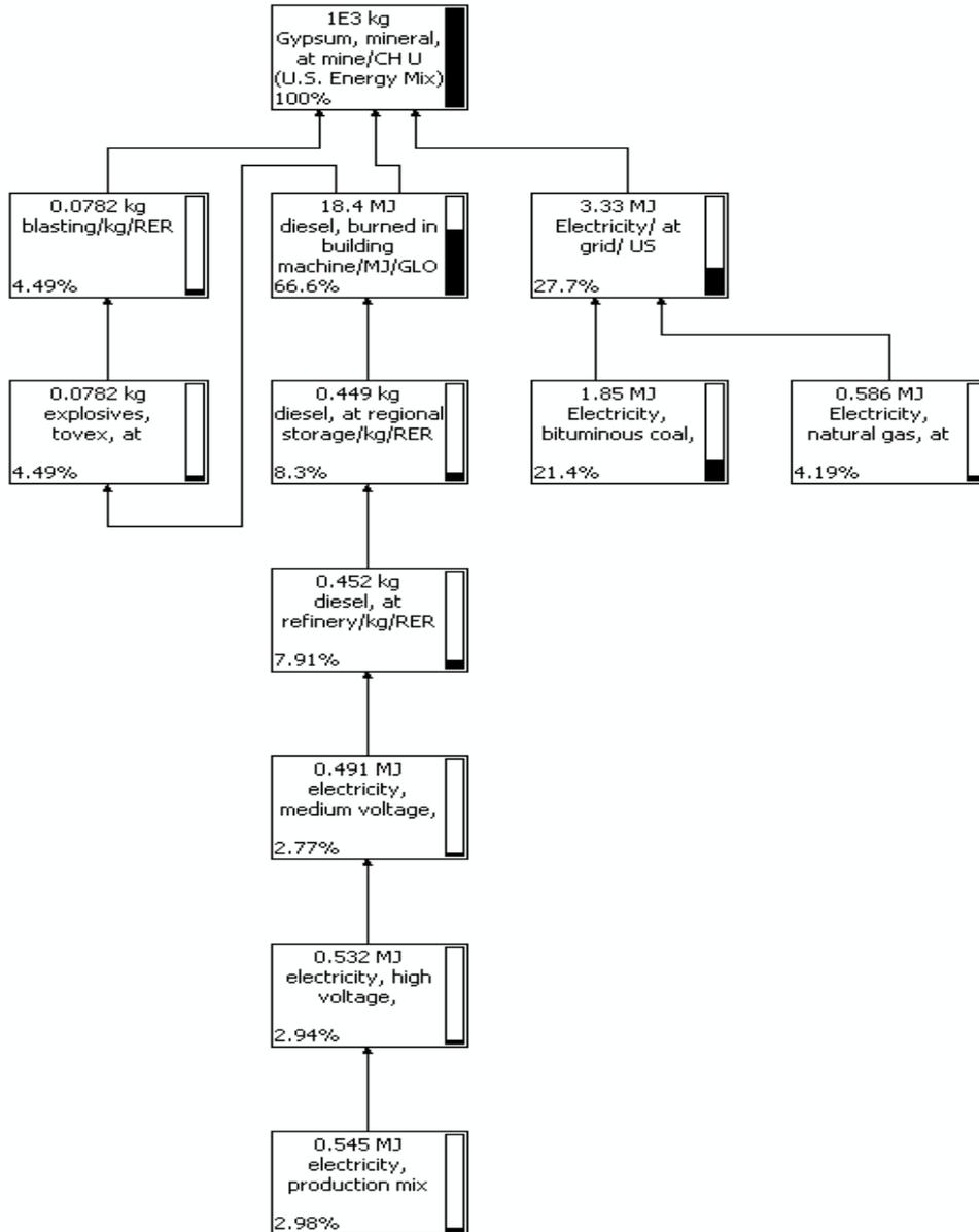
**Figure 2. SimaPro network diagram for mining virgin gypsum.**
