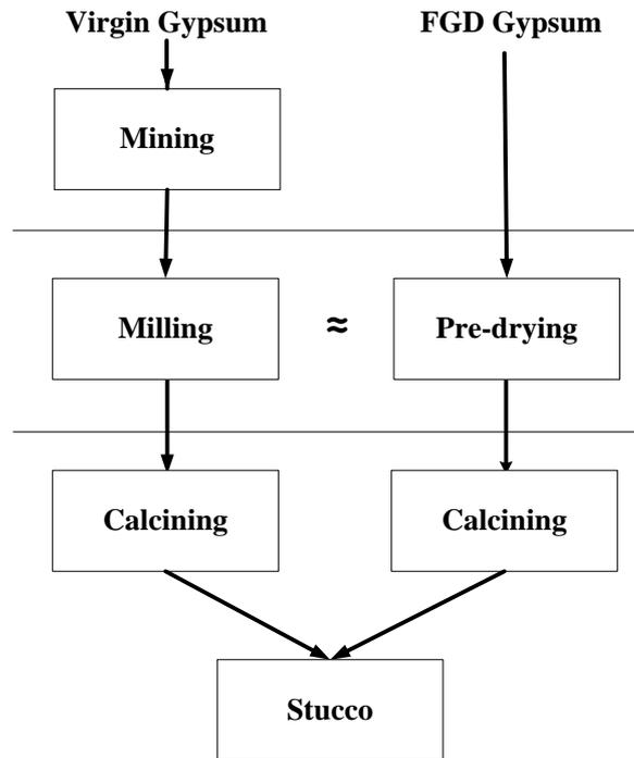
**Figure 1. System boundary for stucco production during wallboard manufacturing using virgin gypsum or FGD gypsum.**
