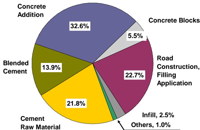
Figure 2. Utilisation of Fly Ash in the Construction Industry and Underground Mining in Europe (EU 15) in 2008.
