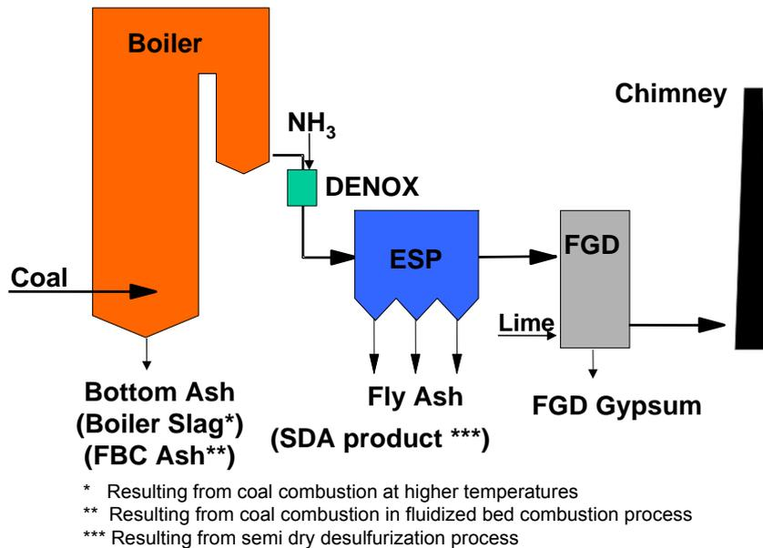
Figure 3 Production of coal combustion products (CCPs) in coal-fired power plants
