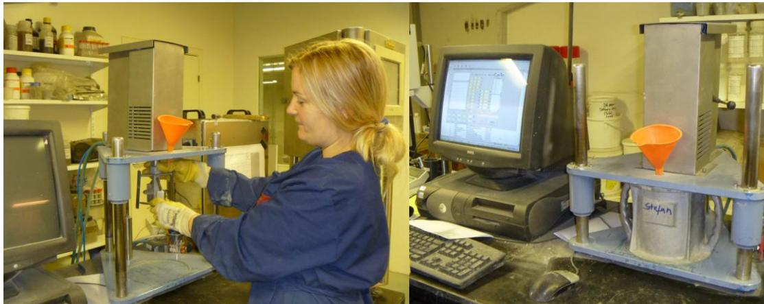
Figure 1. Rheomixer rheology testing equipment. Left: Rheomixer with blade mounting prior to test. Right: Ongoing rheology test with blade inserted in mortar sample.
