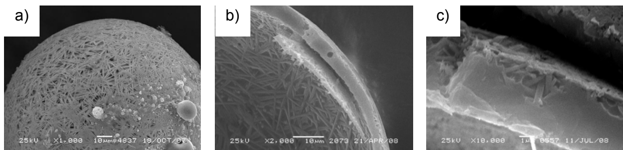
Fig. 3. SEM micrographs of (a) the outer surface and (b) the inner surface and (c) the shell of globules of the narrow fraction NM-M-1A -0.16+0.125
