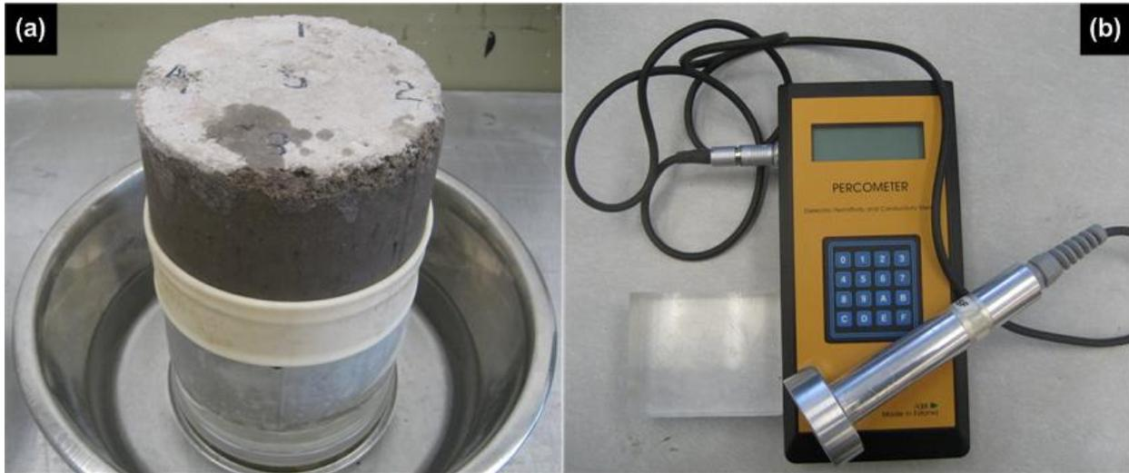
Figure 2. Tube Suction Sample (a) and Percometer (b)
