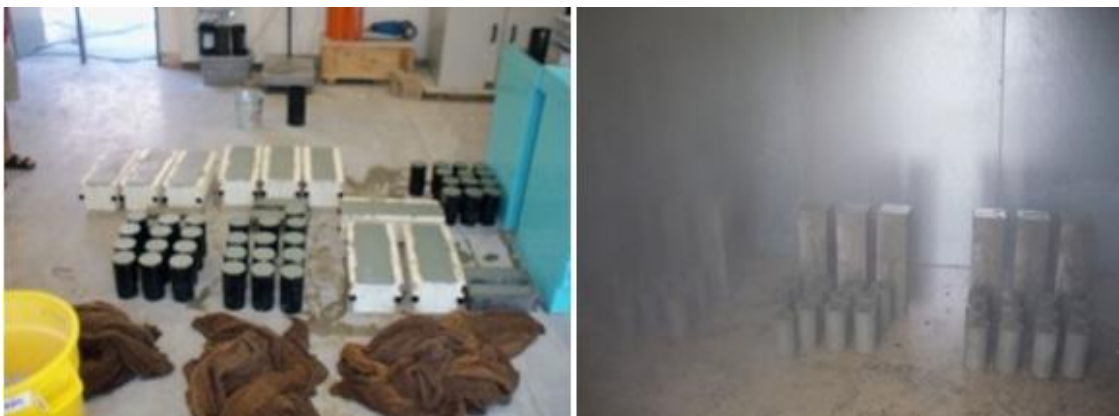
Figure 1 Portion of the test specimens in the lab and in the moisture room
