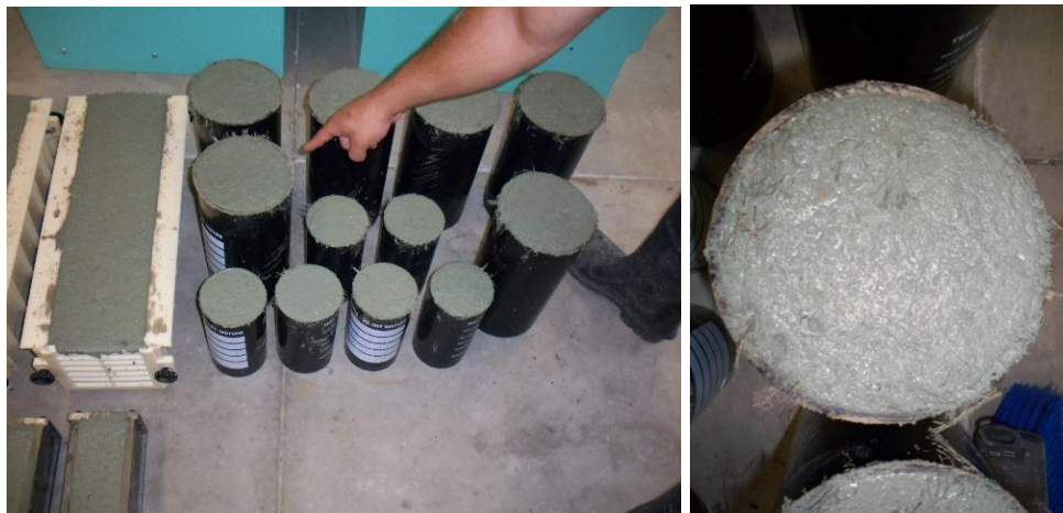
Figure 2 Portion of NXL fiber floated on the surface of the concrete
