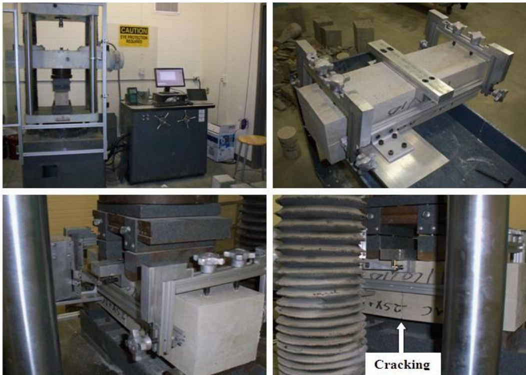
Figure 10 Testing machine, transducers arrangement, and cracking of a beam during ASTM C1609 toughness test
