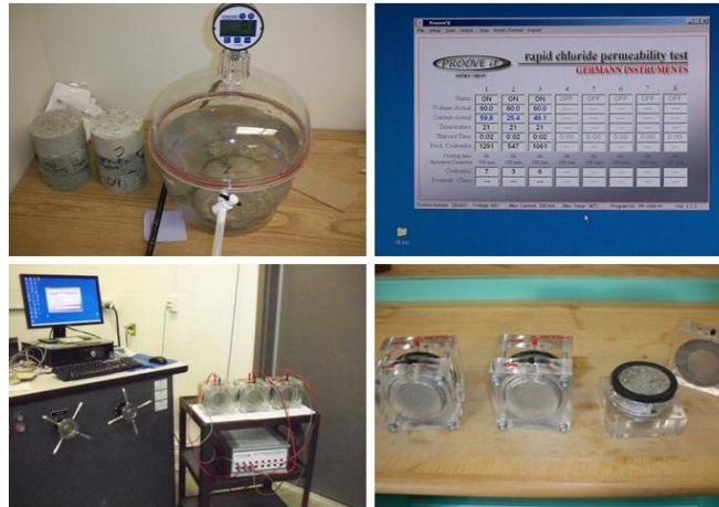
Figure 7 Rapid chloride permeability test and conditioning of the specimens
