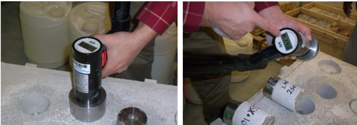
Figure 9 Direct tensile bond strength test equipment
