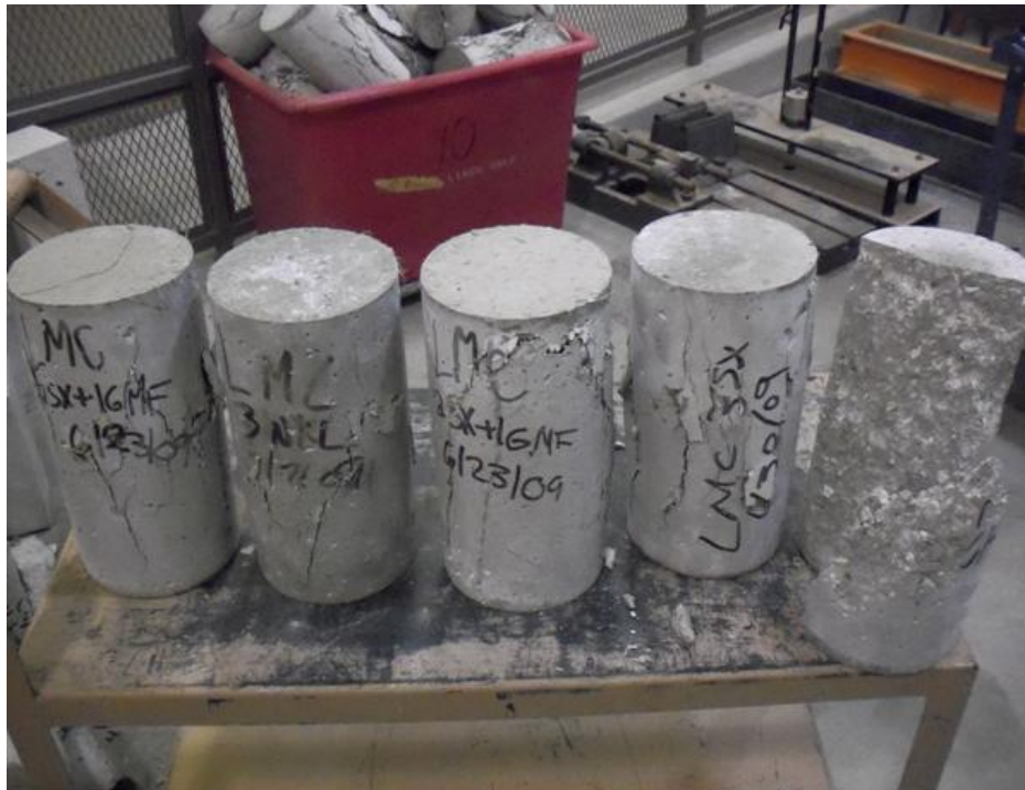
Figure 3 Failure modes of fibrous LMC (left four) and the plain LMC (right)
