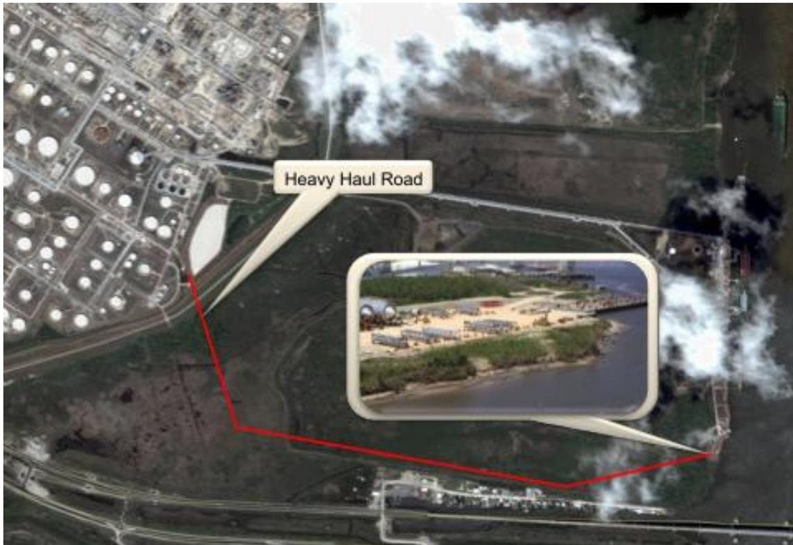
Figure 3: The refinery road was constructed across a dredge pile by stabilizing the dredge spoils and consolidating the underlying soft clays and silts.
