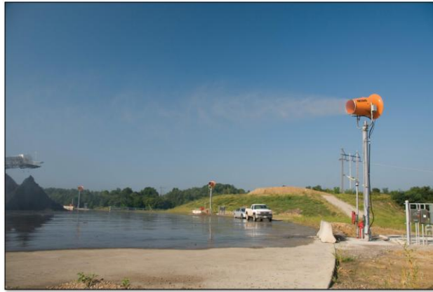
Figure 3: Recent developments in dust suppression include a tower mount design that delivers precise targeting while freeing up ground space for vehicles and other equipment.
