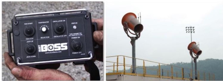
Figure 4: Automated dust suppression units
