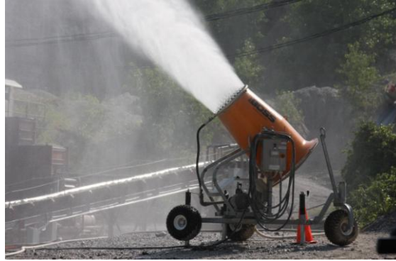
Figure 1: Atomized spray is one of the few suppression technologies capable of delivering dust control by surface wetting AND airborne capture.
