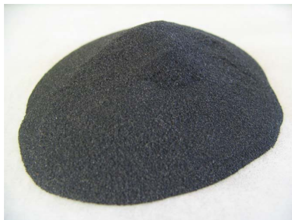
Fig. 2. Picture of ferromagnetic material separated by wet magnetic separator in 200gauss
