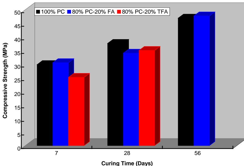
**Figure 3. Compression testing results for 2” mortar cubes for a) 100% portland cement mix (black), b) 80% portland cement with 20% untreated fly ash (blue), and c) 80% portland cement with 20% treated fly ash (red).**
