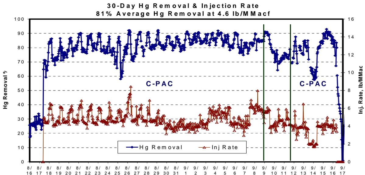
Figure 1. Crawford Unit 7 Mercury Removal & Injection Rates Over 30 Days.
