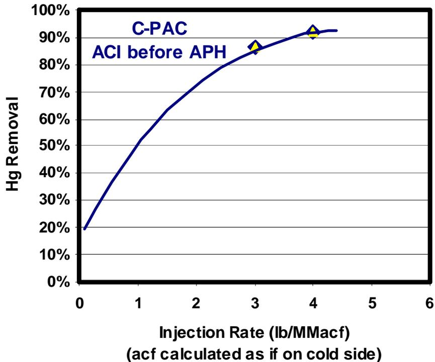
Figure 4. Mercury Removal Rate of C-PAC at Waukegan.
