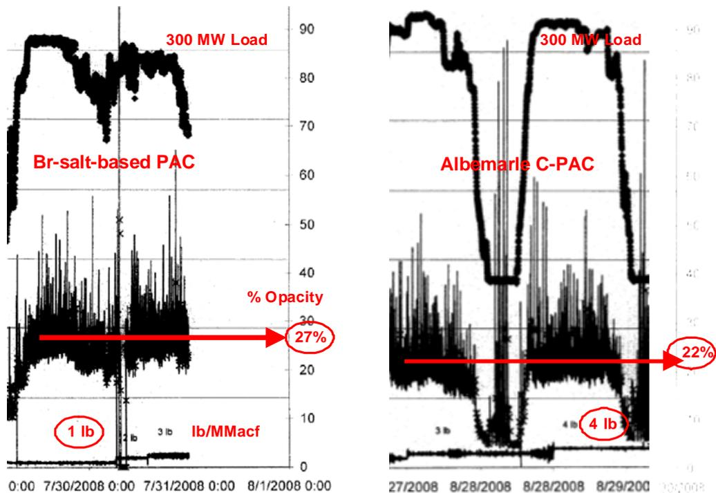
Figure 5. Stack opacity with load with the injection of different sorbents.
