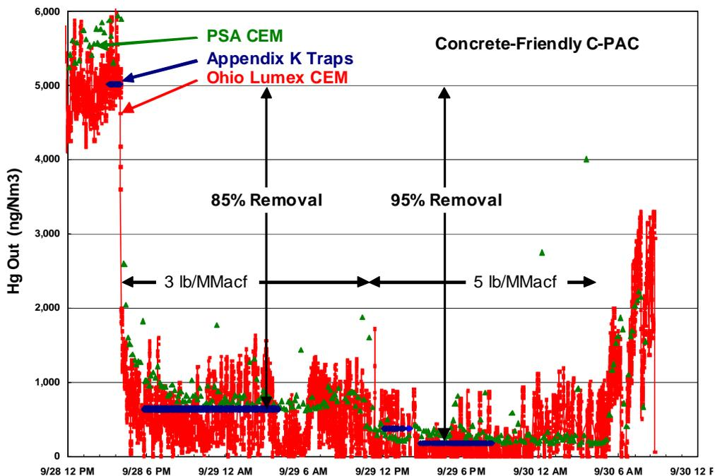
Figure 3. Mercury Removal & C-PAC Injection rate at Corette.
