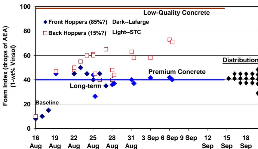
Figure 2. Foam Index of Crawford Fly Ash During a 30-Day C-PAC Injection Trial
