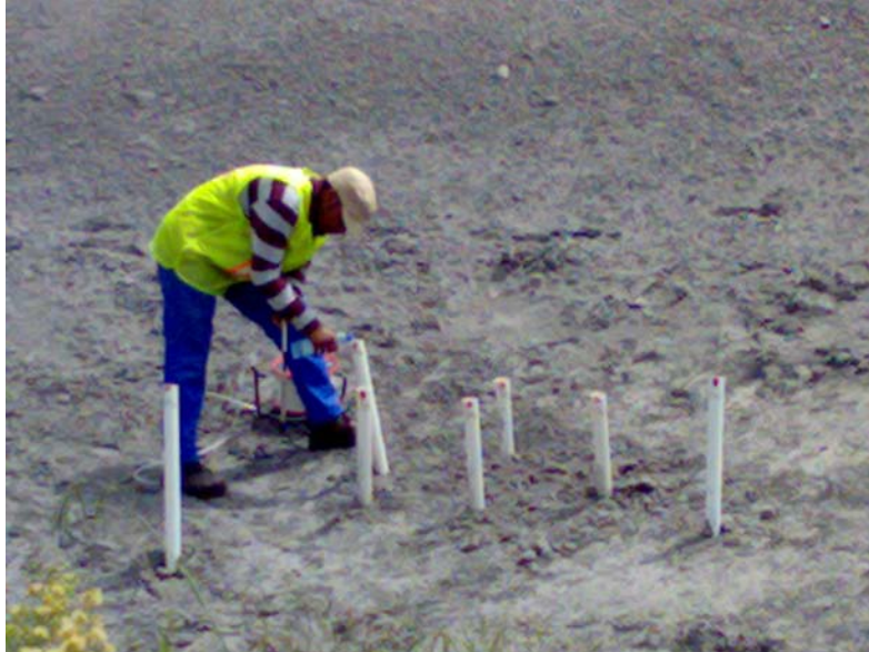
Figure 4 Tracer being injected at a piezometer and immediately monitored, surrounding piezometers were also monitored after tracer injection.
