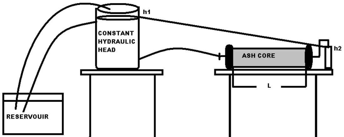
Figure 3 Diagrammatic Sketch of Darcy experimental setup
