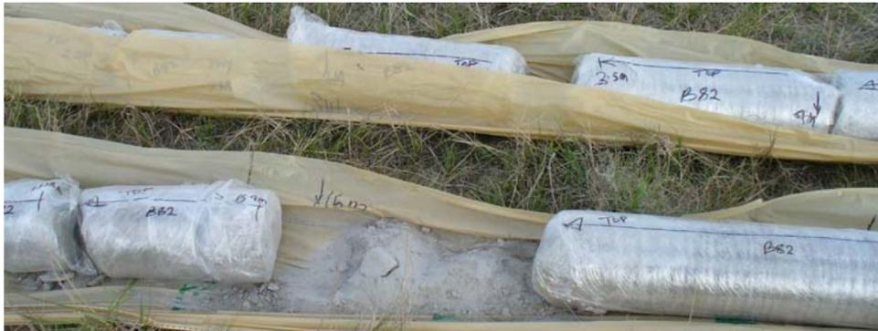
**Figure 2 Air Flush Core collected in the field for Darcy experiment**
