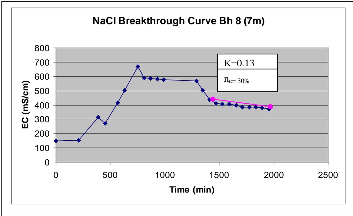
Figure 5 Breakthrough graph used to interpret effective porosity
