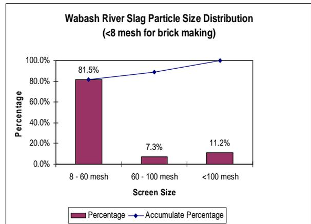
**Figure 2:** Particle size distribution of processed slag (< 8 mesh) for brick making
