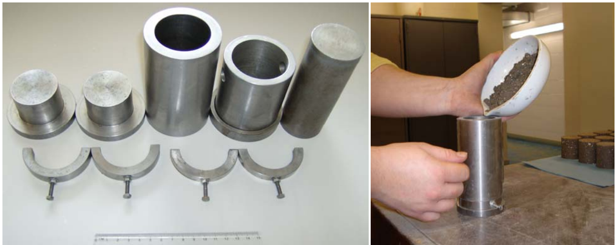
Figure 7. Mould, piston and displacing collars used for the manufacture of specimens 24
