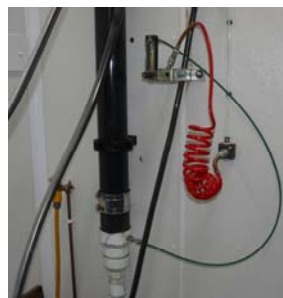
(d) Column froth flotation (same equipment as shown in (c) however, compressed air input used as shown in the photograph)
