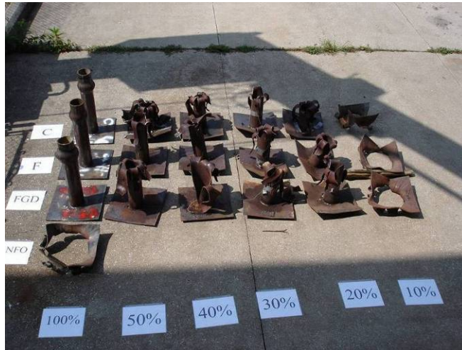
Figure 4. Detonated canisters. Rows are arranged according to CCB type and columns are arranged with decreasing CCB concentrations shown from left to right.
