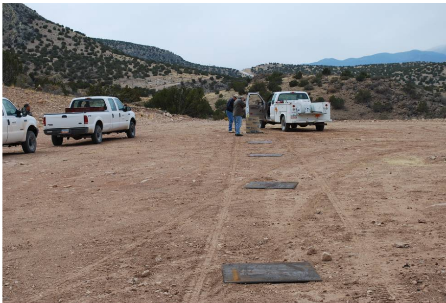
Figure 12. Witness plates prior to detonation of a Sonotube cylinder that was loaded with 140-kg charges as shown near the truck in back-center.
