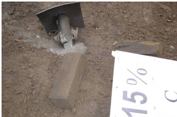
Figure 6. Canister remnant following detonation of a 15% FAC-coated charge (note the large quantity of unexploded prills on ground).
