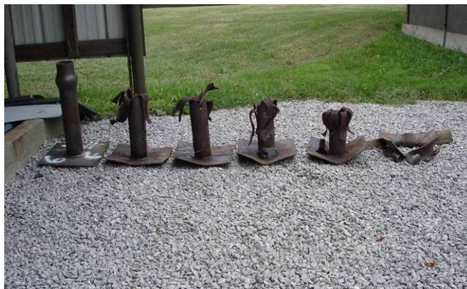
Figure 5. Detonated-canister remnants for the FAF-coated AN. l-r, 100, 50, 40, 30, 20, & 10%-coated charges.
