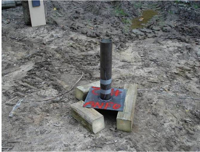
Figure 3. A detonation canister prior to detonation.
