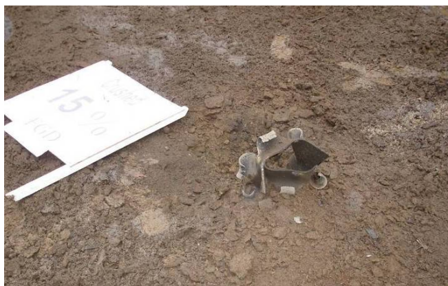
Figure 10. Base-plate remnant following detonation of a crushed sample coated with 15% FGD.
