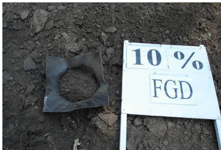
Figure 7. Canister remnant following detonation of AN coated with 10% FGD byproduct.
