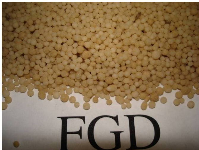
Figure 2. AN prills coated with a 20% FGD byproduct in a drum roller.
