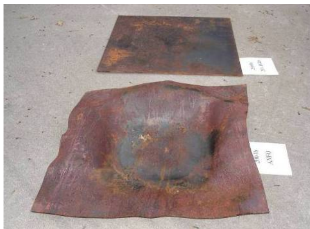
Figure 11. Witness plates following detonation of 90-kg charges of 100% AN (front) and 20% FGD-coated AN (back).
