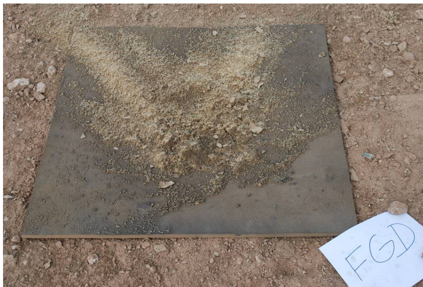
Figure 14. Witness plate following detonation of FGD-coated AN showing unexploded sample remaining after detonation.
