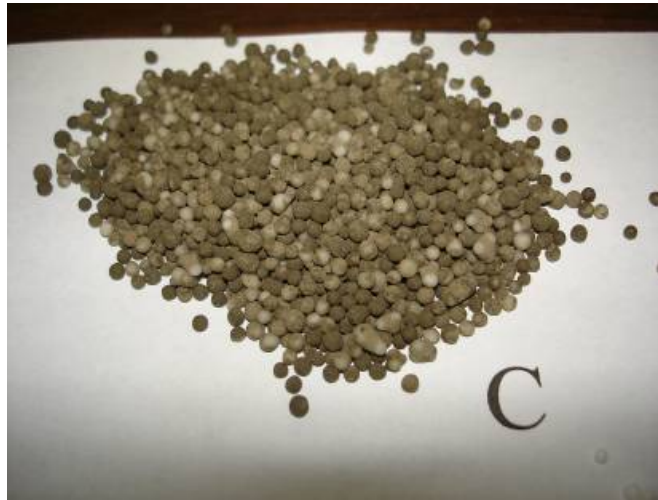
Figure 1. AN prills coated with 25% FAC in a disk pelletizer.
