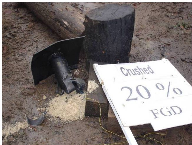
Figure 9. Photograph of the containment-canister remnant following detonation of a crushed sample of 20%-FGD-coated AN. Note the presence of unexploded material spilled onto the ground.
