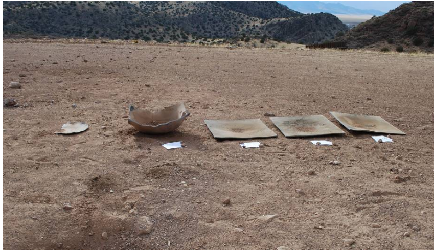
Figure 13. Witness plate remnants following detonation of 140-kg charges of (left to right) 100% ANFO, calcium ammonium nitrate, and ammonium nitrate coated with 21.7% FAF, 20.7% FGD, and 21.0% FAC, respectively.
