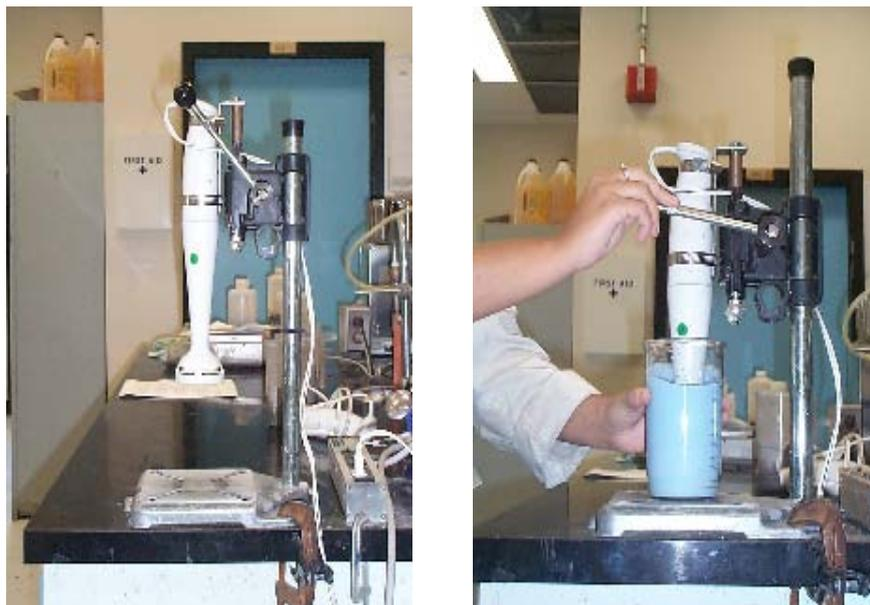
**Figure 1:** Illustration of paste mixing device for air entrainment and fluidity measurements.
